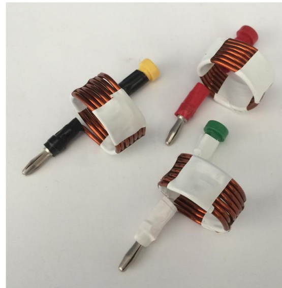
(c) Three air core inductors designed as auxiliary inductors.
