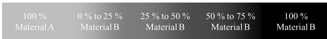
Figure 1-3. A stepwise FGM with three intermediate regions, each implementing a continuous gradient between the discrete boundaries.
