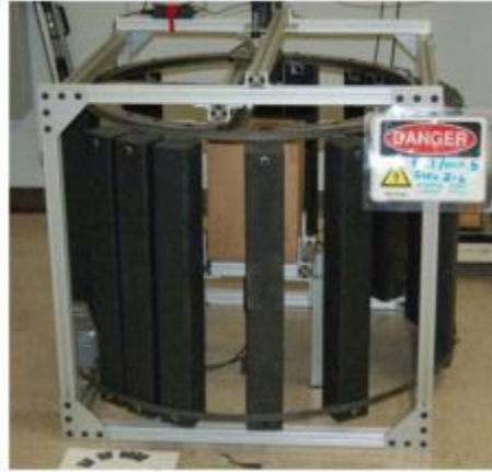
Figure 4. Time-encoded fast-neutron imager. (Marleau, et al., 2011) ©IEEE 2011.
