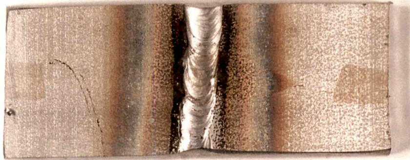
Figure 4.26: Photograph of 304L/316L weldment (as-welded, non-creviced). Tested in abiotic solution that simulates the Arizona well-water system.
