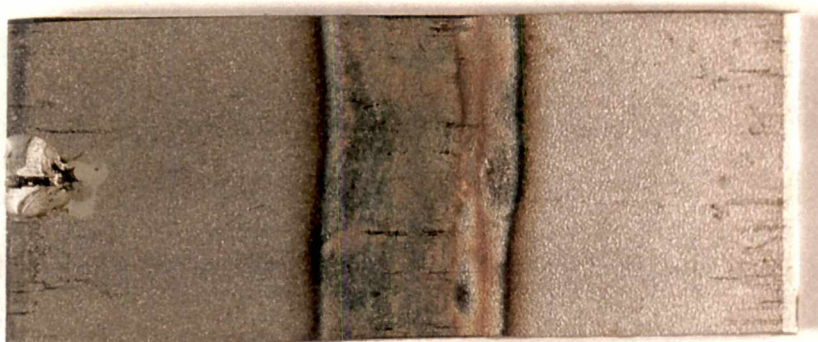
Figure 4.21: Photograph of AL-6XN weldment, as-welded and non-creviced. Tested in abiotic solution that simulates the Delaware Bay site water.
