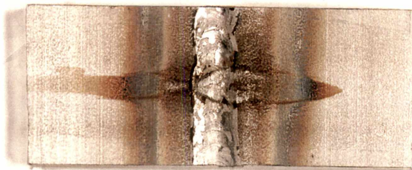
Figure 4.30: Photograph of 304L/316L weldment (as-welded, creviced). Tested in abiotic solution that simulates the Tennessee River fresh-water system.
