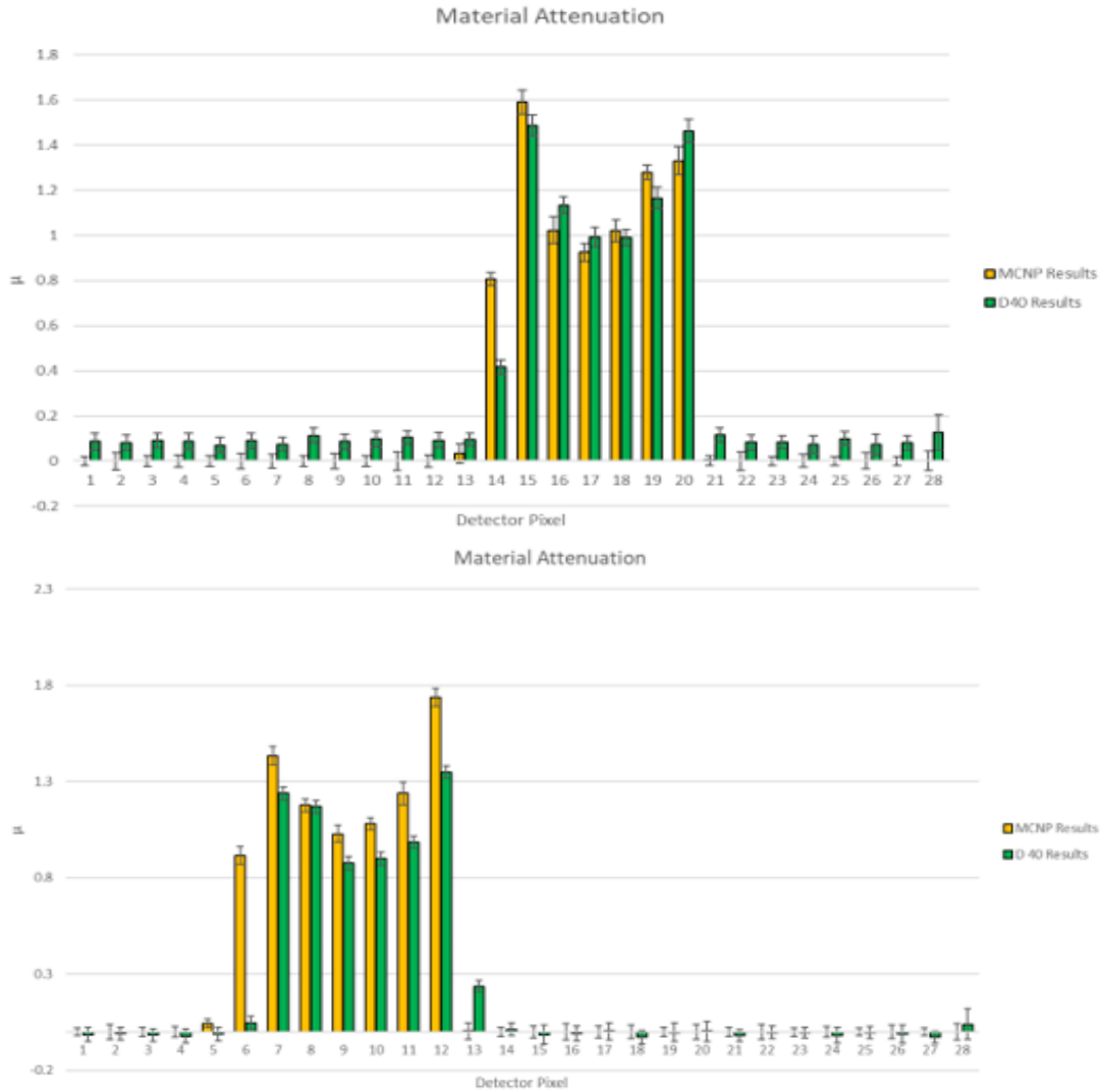
Figure 4.6. DT-detector equidistant, offset top (5cm) and offset bottom (10cm) steel attenuation profile
