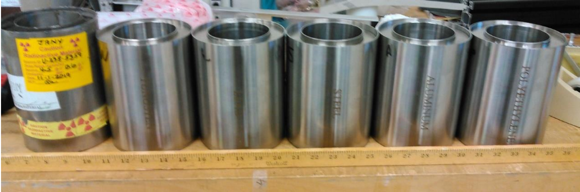
Figure 4.1. Material canisters made of depleted uranium (DU), tungsten, lead, steel, aluminum, and polyethylene, pictured from left to right.
