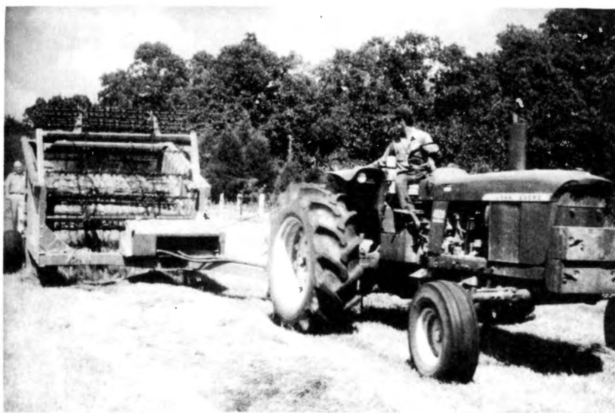
Figure 2. Roll baler packaging a bale of hay.
