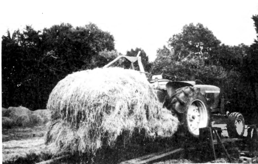
Figure 5. Roll bale handled by tractor-stackmover combination and weighed on portable field scales.
