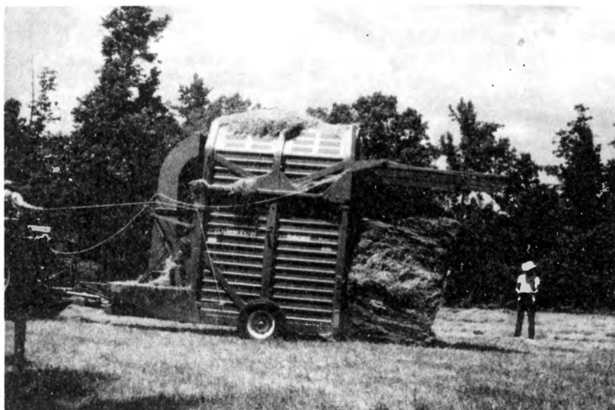
Figure 3. Stacker unloading to complete the packaging process.
