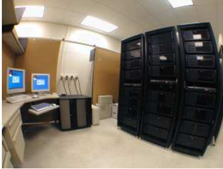
Figure 2.4: A lab built parallel machine consisting of 2 server nodes and 24 computing nodes. Photo courtesy of J. D. Birdwell [27].
