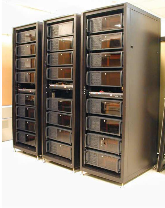
Figure 1.2: A parallel cluster of 24 computing nodes built in the LIT lab. Photo courtesy of J. D. Birdwell [27].
