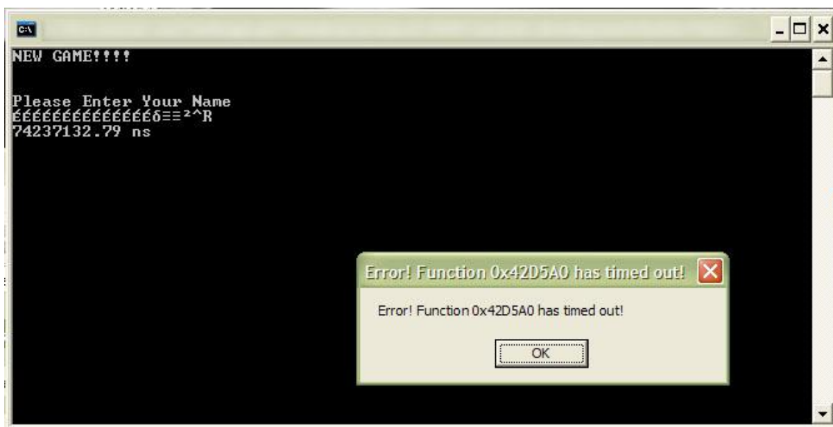
Figure 6.9: The watchdog timer detects that Foo() never returns and alerts the user.
