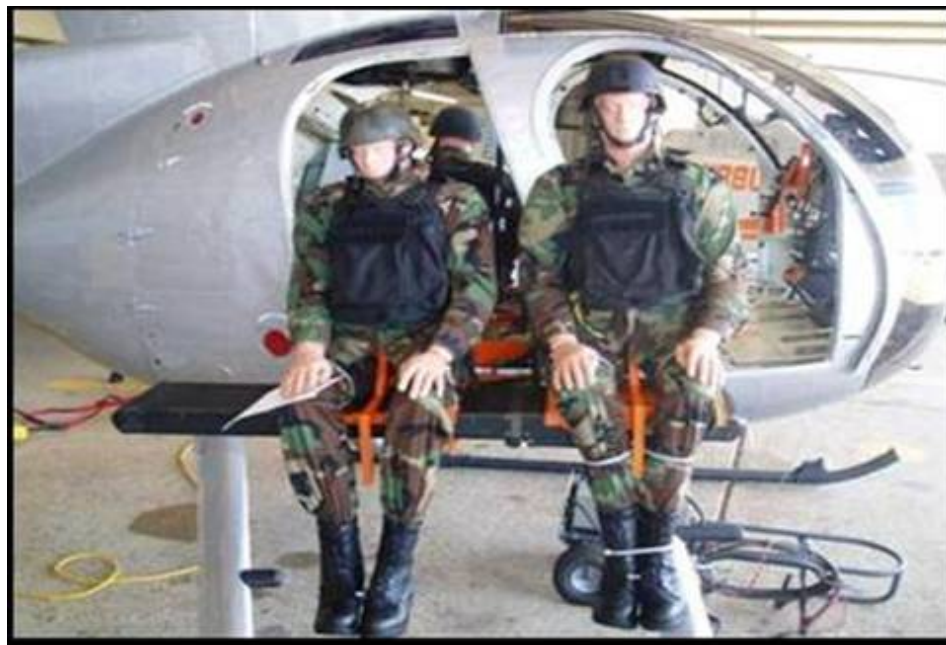
Figure 4. Manikins Seated on EPS
