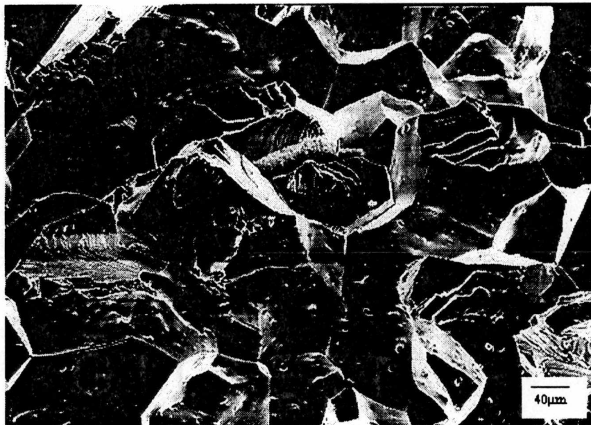
Figure 53: Fracture surface of 1000°C furnace oxide sample of FAL slow strain-rate specimen tested at -1500 mV SHE.
