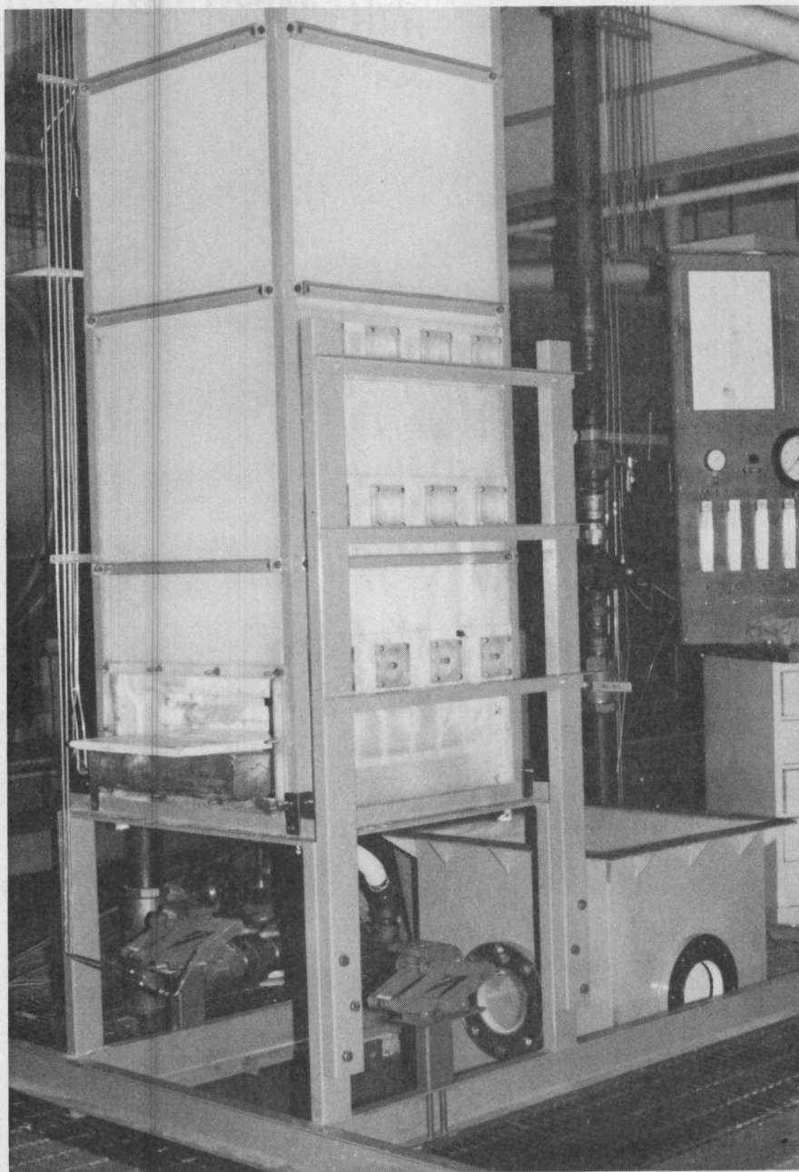
Figure 5.5. Plenum Box Removed from the Bed Section.
