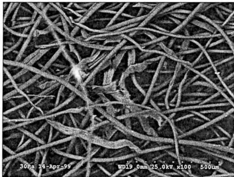
Figure 4.12 SEM Image Showing Disintegration of Bond (Final Stage)
