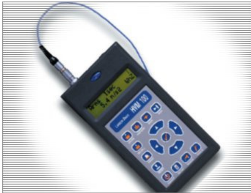
Figure 4.7: Human Vibration Meter
