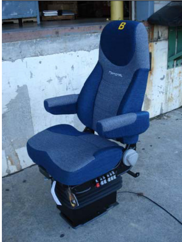
Figure 4.4: Standard Commercial Vehicle Seat Model 2000 used for test
