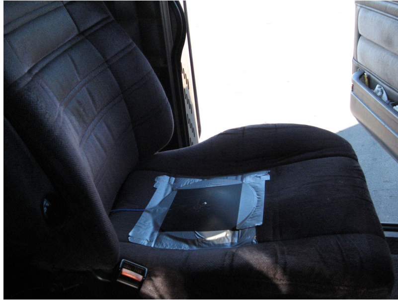
Figure 4.6: Seat Pad containing triaxial accelerometer
