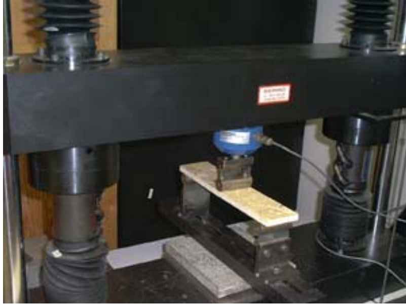
Figure 4. The stiffness test is applied to a specimen. See http://forest.mtu.edu/research/woodprotection/research/mechanical.html
