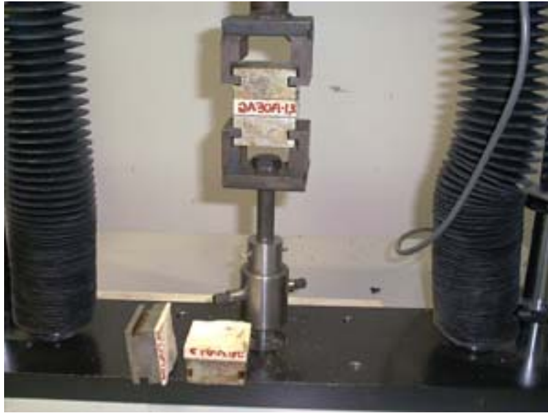
Figure 3. Applying tensile load to internal bond specimen. Also shown is failed specimen. http://forest.mtu.edu/research/woodprotection/research/mechanical.html
