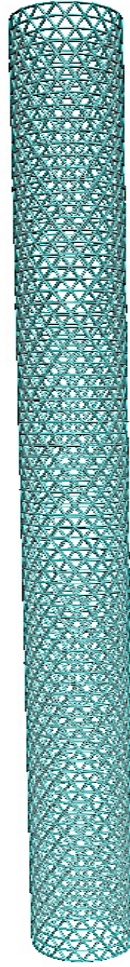
Figure 26 | Initial configuration for a cylindrical membrane with 1596 particles (84 layers with 19 particles in each layer)
