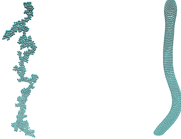
Figure 33 | Configurations of confined fluid membranes with \kappa = 0 (left) and 1000 (right) after 2 \cdot 10^6 MCS.
