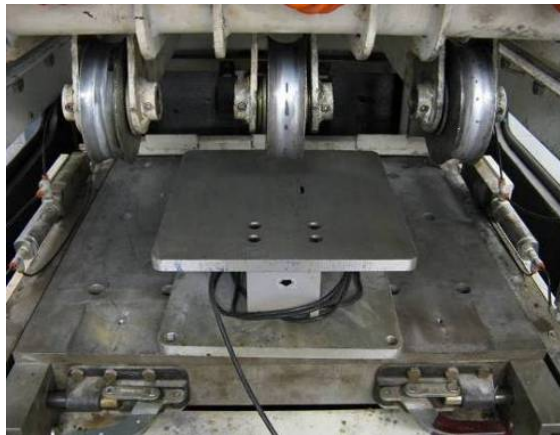
(b) Movable wheels and load cell
