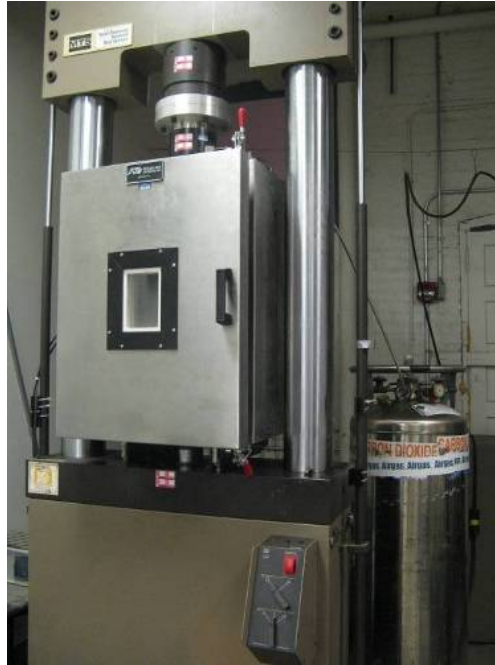
Figure 4.15 MTS loading system with environmental chamber
