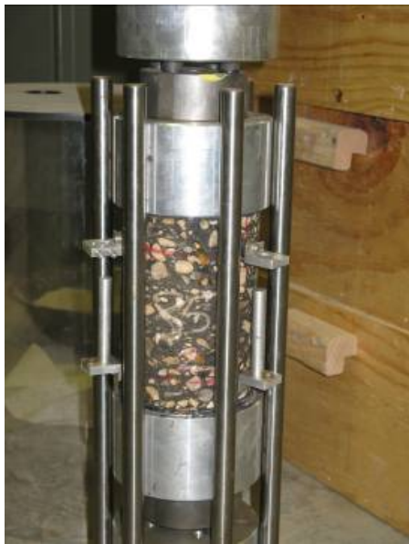
(c) Specimen and loading plates alignment
