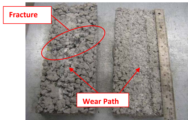
(b) The damage on specimen
