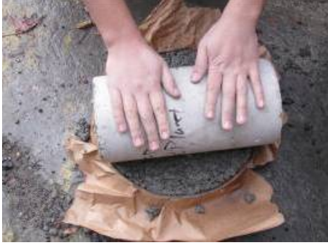
(a) Rolling compaction
