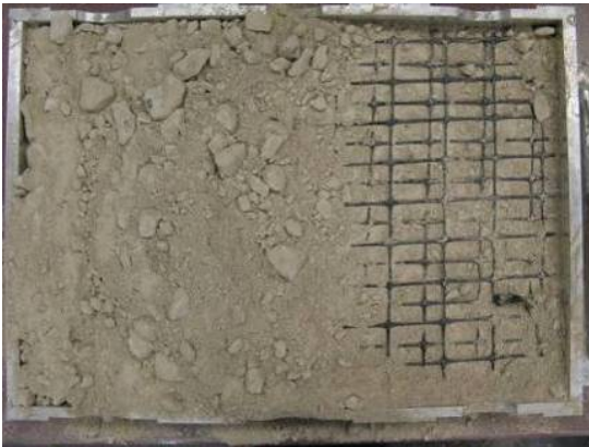
(a) Base course with geogrids reinforced
