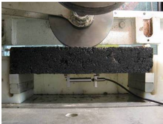
(c) Loaded wheel viscoelastic test setup
