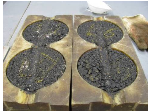
(b) Samples after rutting test
