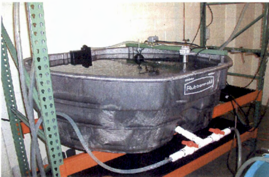
Figure 3. Head tank design with water lines.
