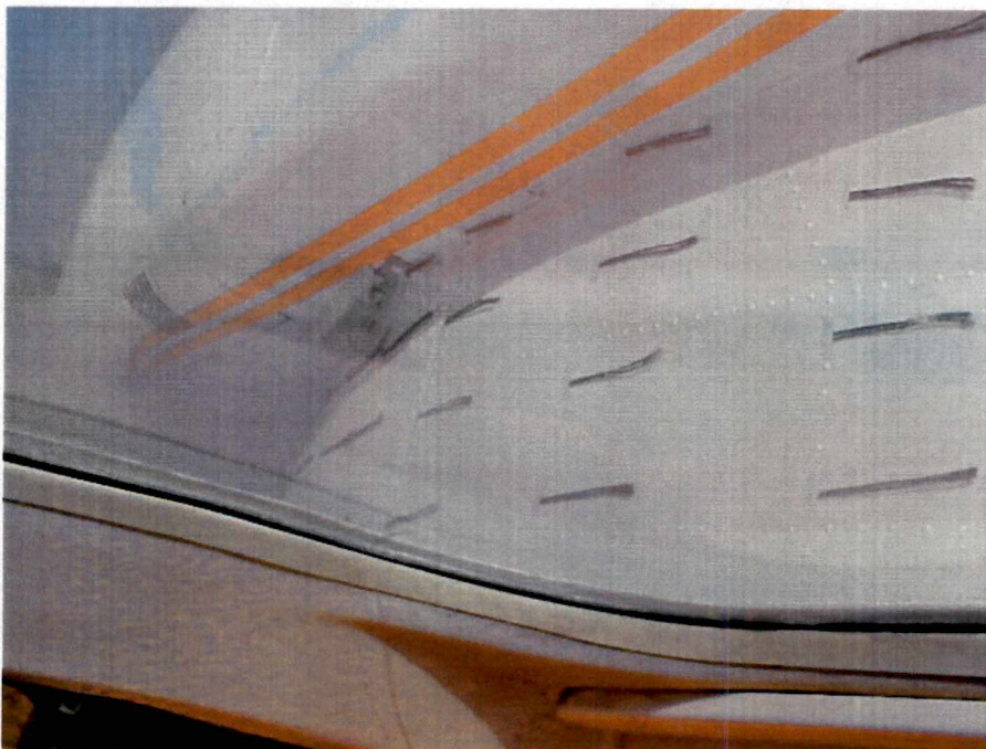
Figure 6.16b. Flow Visualization between Fuselage and Right Nacelle towards Leading Edge at 110 Knots - Strake Configuration
