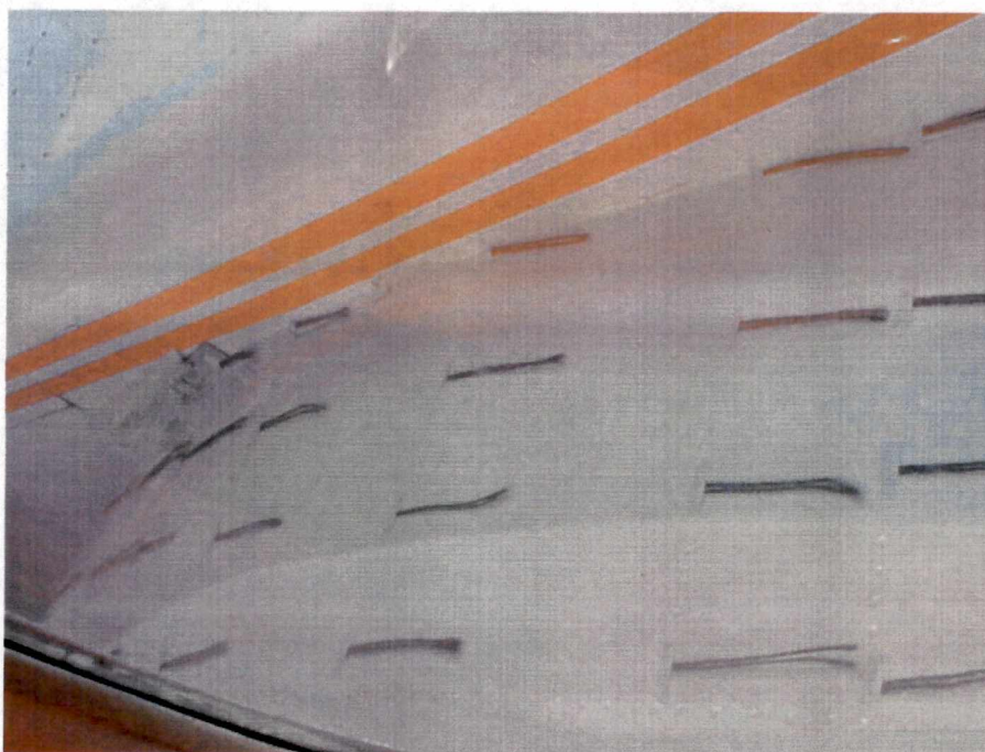
Figure 6.14b. Flow Visualization between Fuselage and Right Nacelle towards Leading Edge at 130 Knots - Strake Configuration
