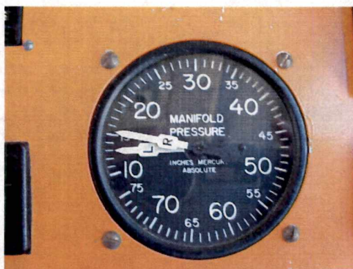
Figure 3.8. Manifold Pressure Indicator for Center Left Console in Piper Navajo
