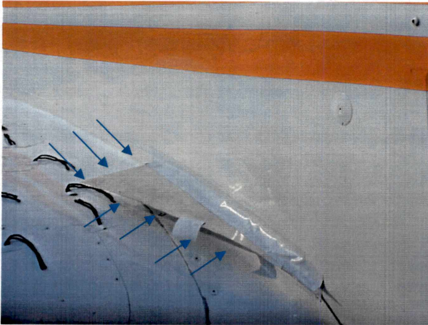
Figure 4.1a. Right Fuselage Strake Mounted to Right Fuselage (blue arrows point to strake)
