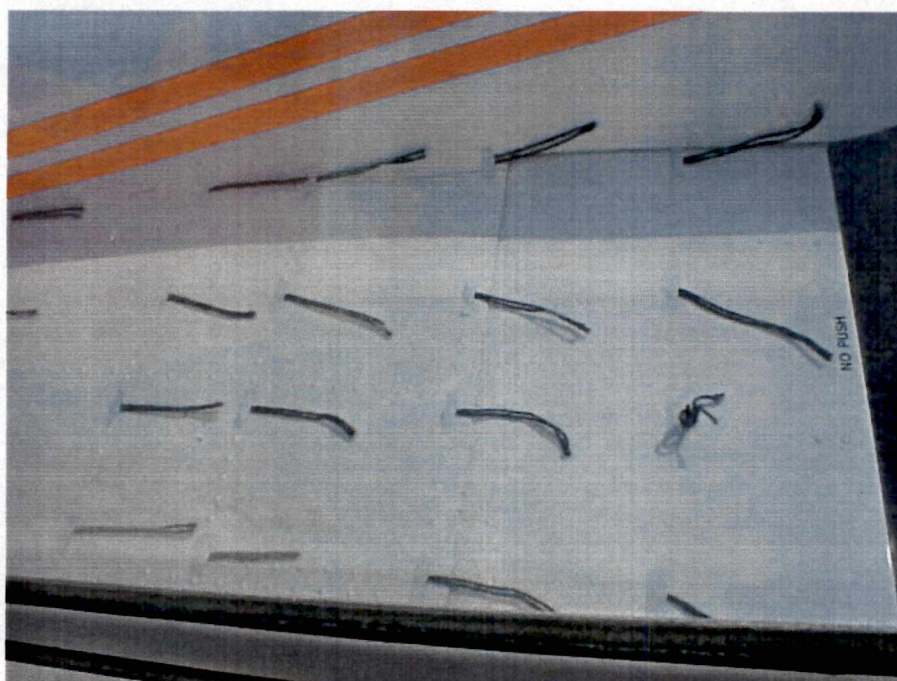
Figure 6.18d. Flow Visualization at Trailing Edge of Right Wing at 90 Knots - Strake Configuration
