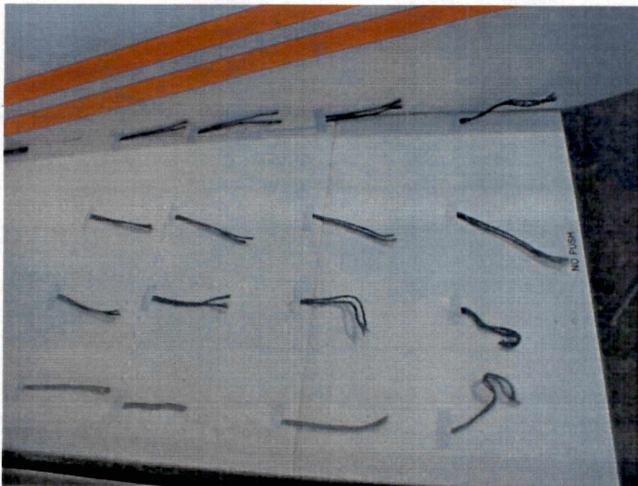
Figure 6.19d. Flow Visualization of Trailing Edge of Right Wing at 80 Knots - Strake Configuration
