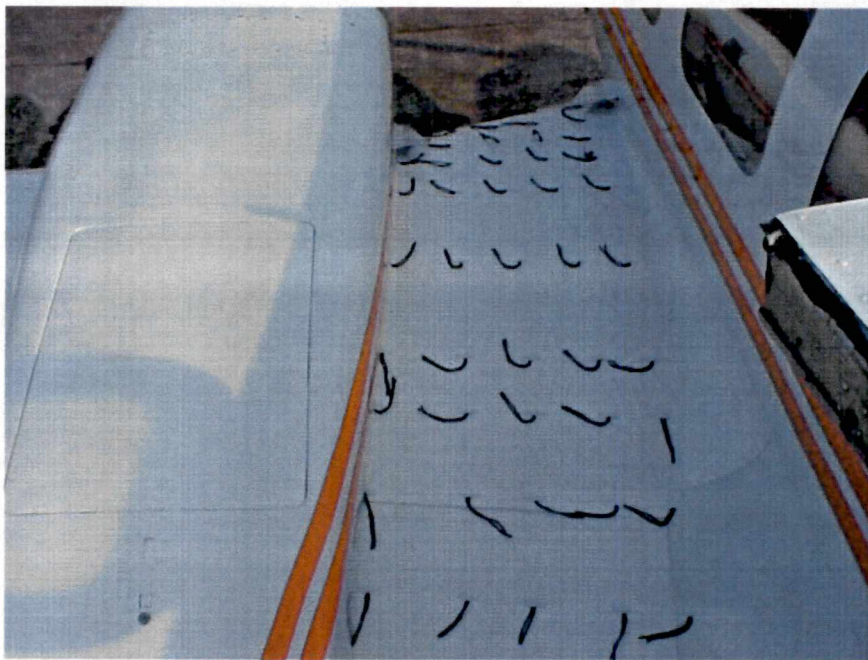
Figure 4.2b. Left Wing with Tufts and Strakes Mounted
