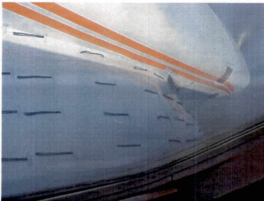
Figure 6.16f. Flow Visualization between Fuselage and Left Nacelle towards Leading Edge at 110 Knots - Strake Configuration
