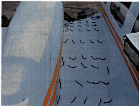
Figure 3.4b. Tufts on Left Inboard Wing between Nacelle and Fuselage
