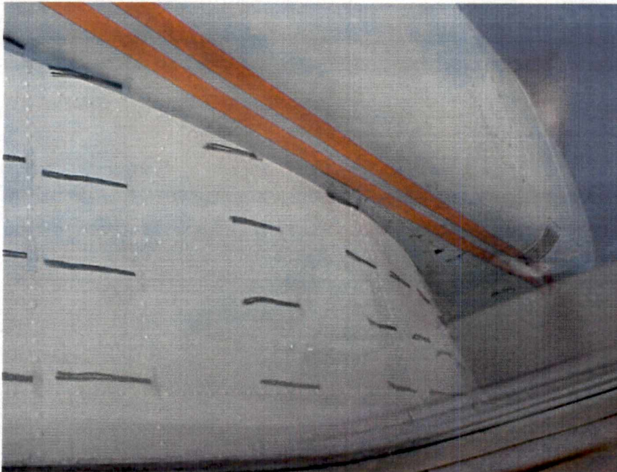
Figure 6.16e. Flow Visualization between Fuselage and Left Nacelle towards Leading Edge at 110 Knots - Baseline Configuration
