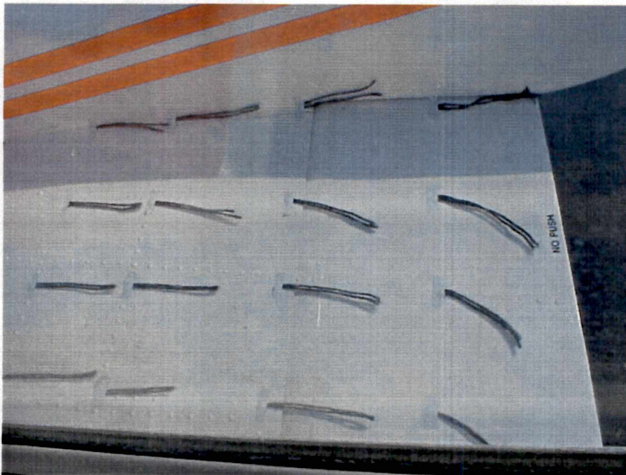
Figure 6.15d. Flow Visualization at Trailing Edge of Right Wing at 120 Knots - Strake Configuration
