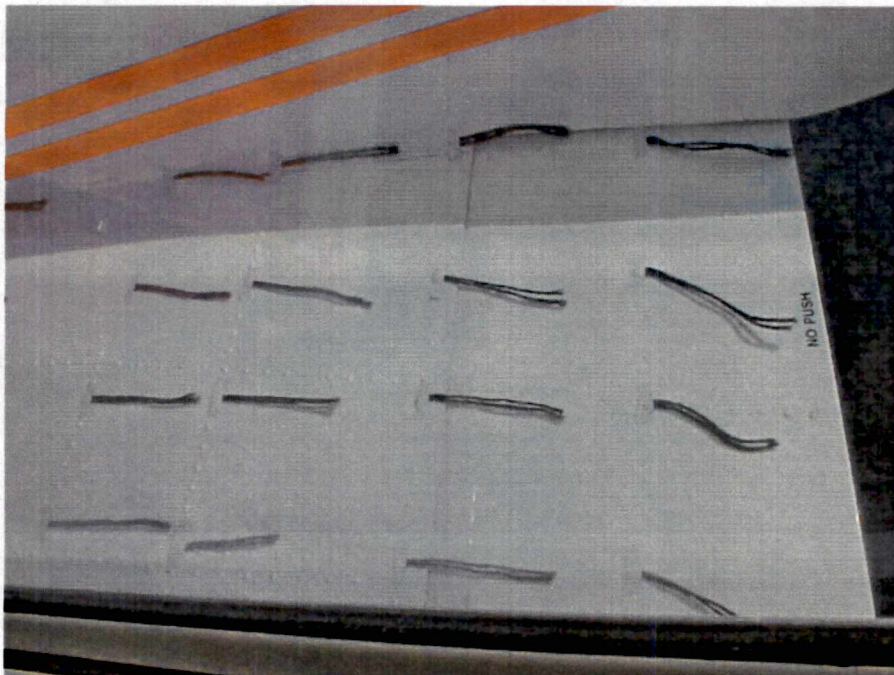
Figure 6.16d. Flow Visualization at Trailing Edge of Right Wing at 110 Knots - Strake Configuration
