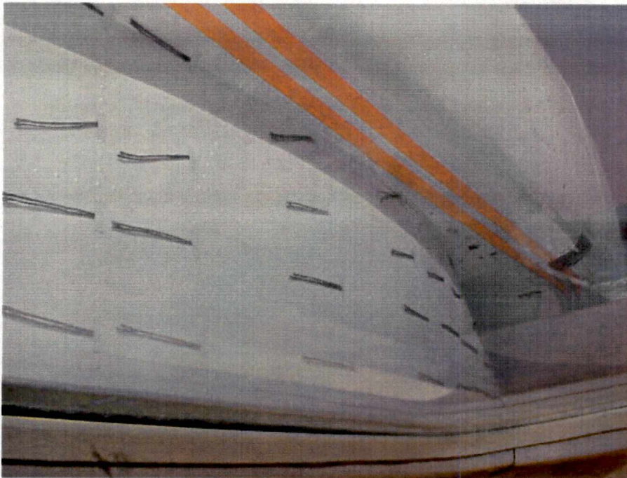
Figure 6.19e. Flow Visualization between Fuselage and Left Nacelle towards Leading Edge at 80 Knots -Baseline Configuration
