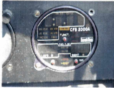
Figure 3.10. Fuel Quantity Indicator in Cockpit of Piper Navajo
