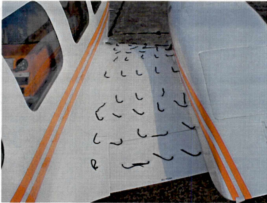
Figure 4.2a. Right Wing with Tufts and Strakes Mounted
