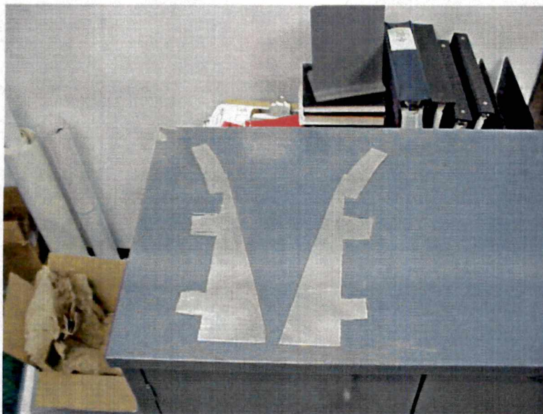
Figure 3.3c. Outboard Nacelle-Wing Intersection Strakes
