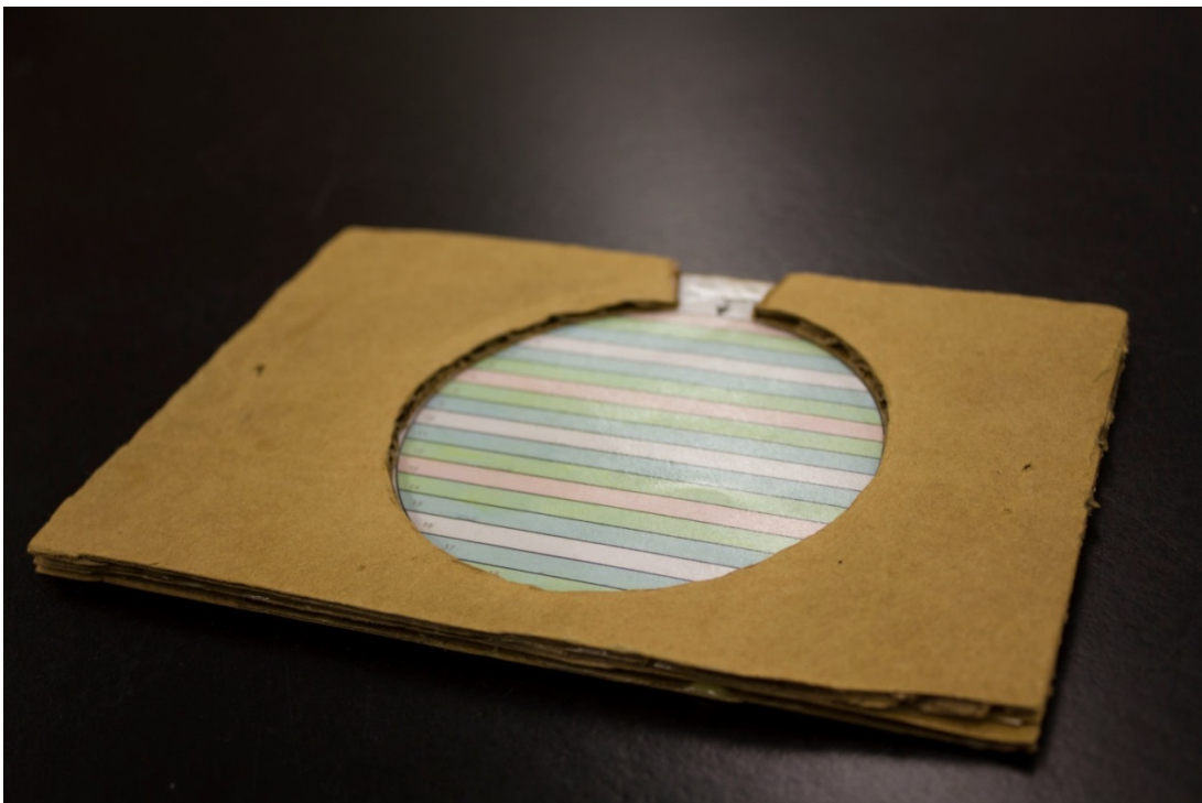
Figure 4.5. Side view of petri dish holder showing the walls that hold the dish in place.
