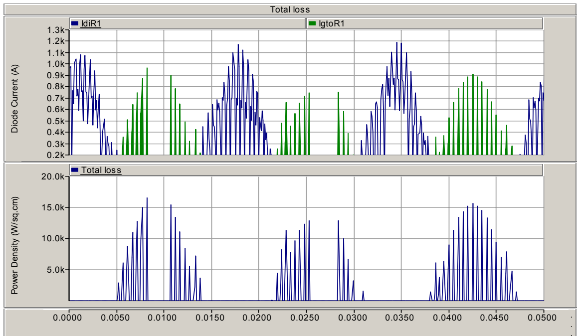
Figure 4-16: Loss profile and diode current for SiC GTO (373 K)
