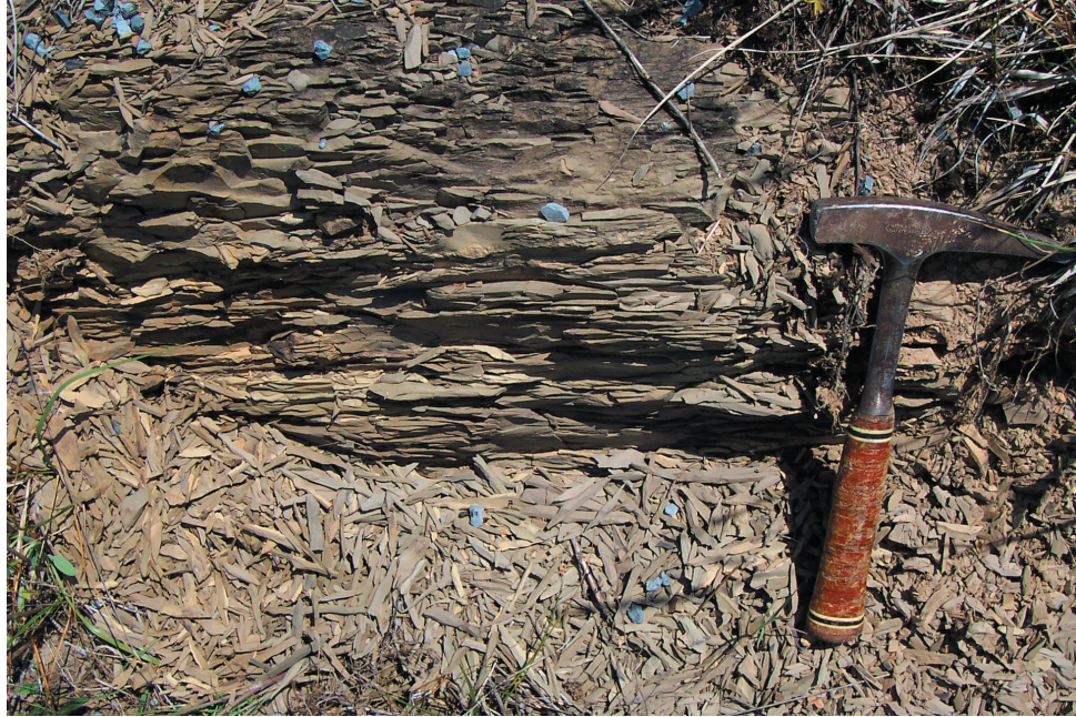
Figure 2-5. Penciled, non-calcareous, fissile Nolichucky Shale. Orientation of pencils is 021^{\circ} , 17^{\circ} NE. Located northeast of Ottinger Shelton Chapel. (Hammer is ~ 12 in long.)
