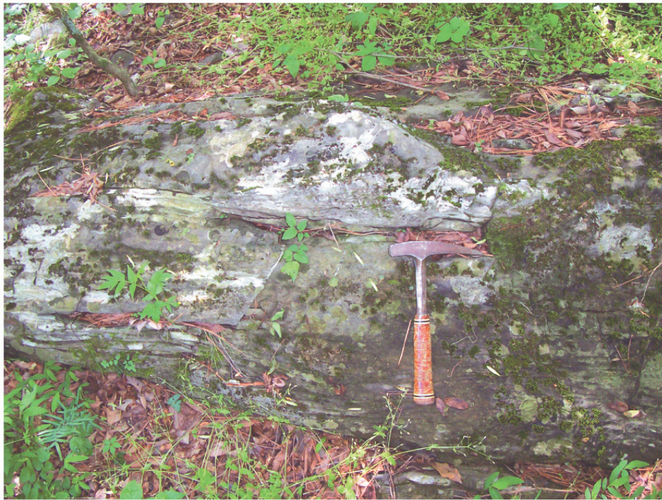
Figure 2-12. Typical outcrop of Kingsport Formation limestone. The outcrop is located near Luther Memorial Church, TN. Hammer head is parallel to bedding plane. (Hammer is ~ 12 in. long.)
