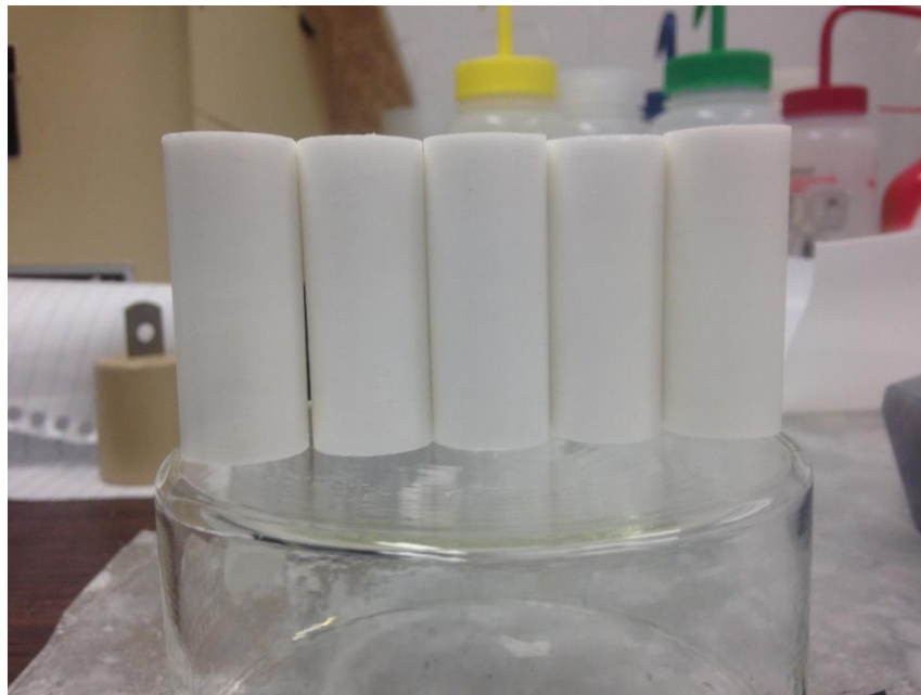
Figure 27. Uniaxial test specimen cylinders, aspect ratio 2.5.
