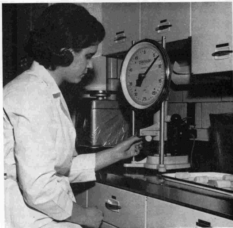
Figure 11. A graduate student in food science is determining the force required to shear a core of beef from a rib roast to obtain an index of its tenderness.
