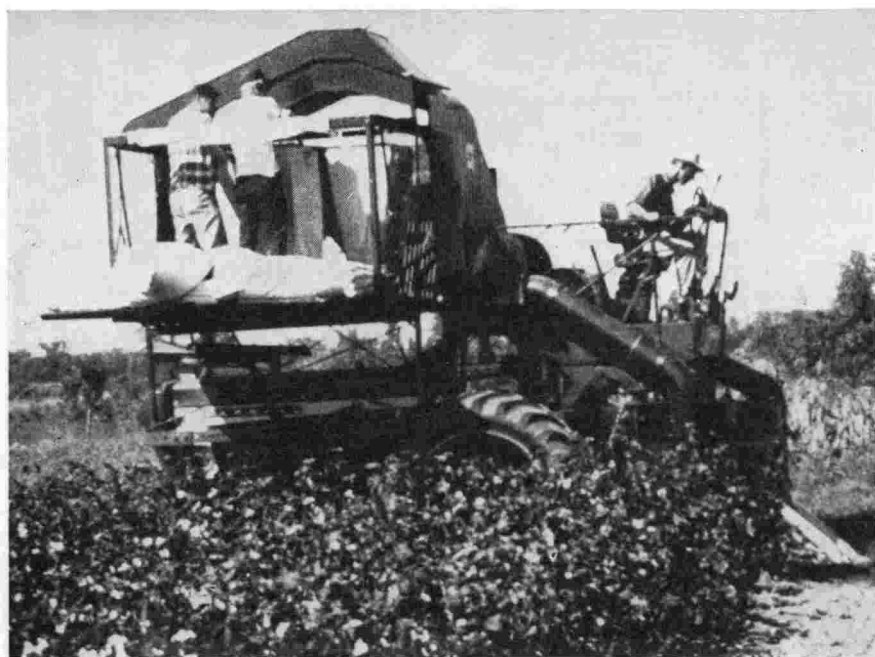
Figure 2. Harvesting cotton plots with one-row spindle picker equipped with a special sacking attachment for collecting samples.
