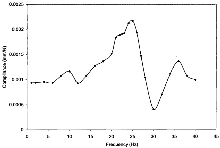
Figure A126: Specimen 10 flexion angle intact compliance graph at 800N preload, 0.04 mm amplitude
