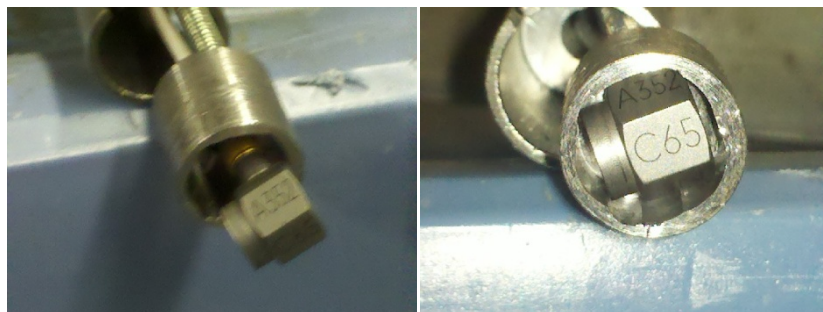
Figure 14: Accelerometer Placed in Casing Prior to Testing
