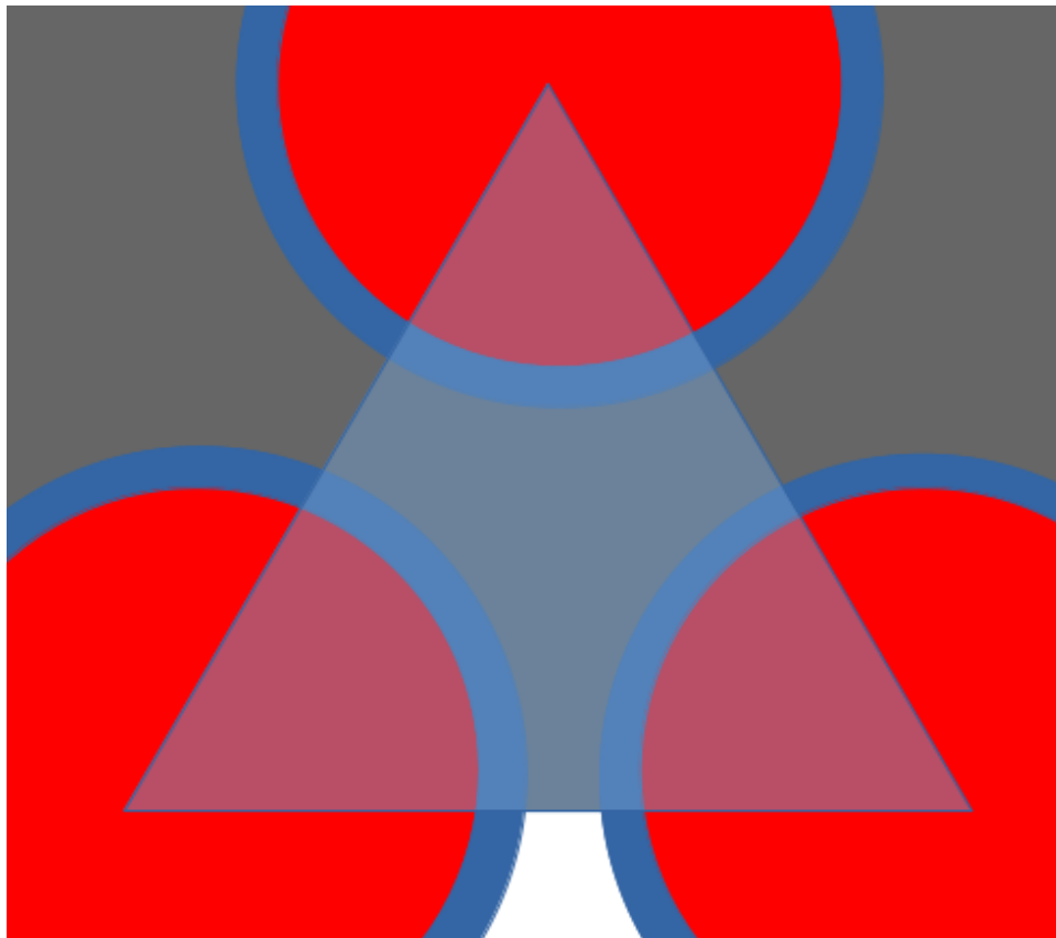
Figure 5.2: Combined Heat Pipe and Fuel Unit Cell Equivalent
