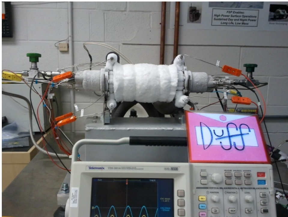
Figure 8.6: First operation of Buzz converters on test stand, 90 days prior to experiment
