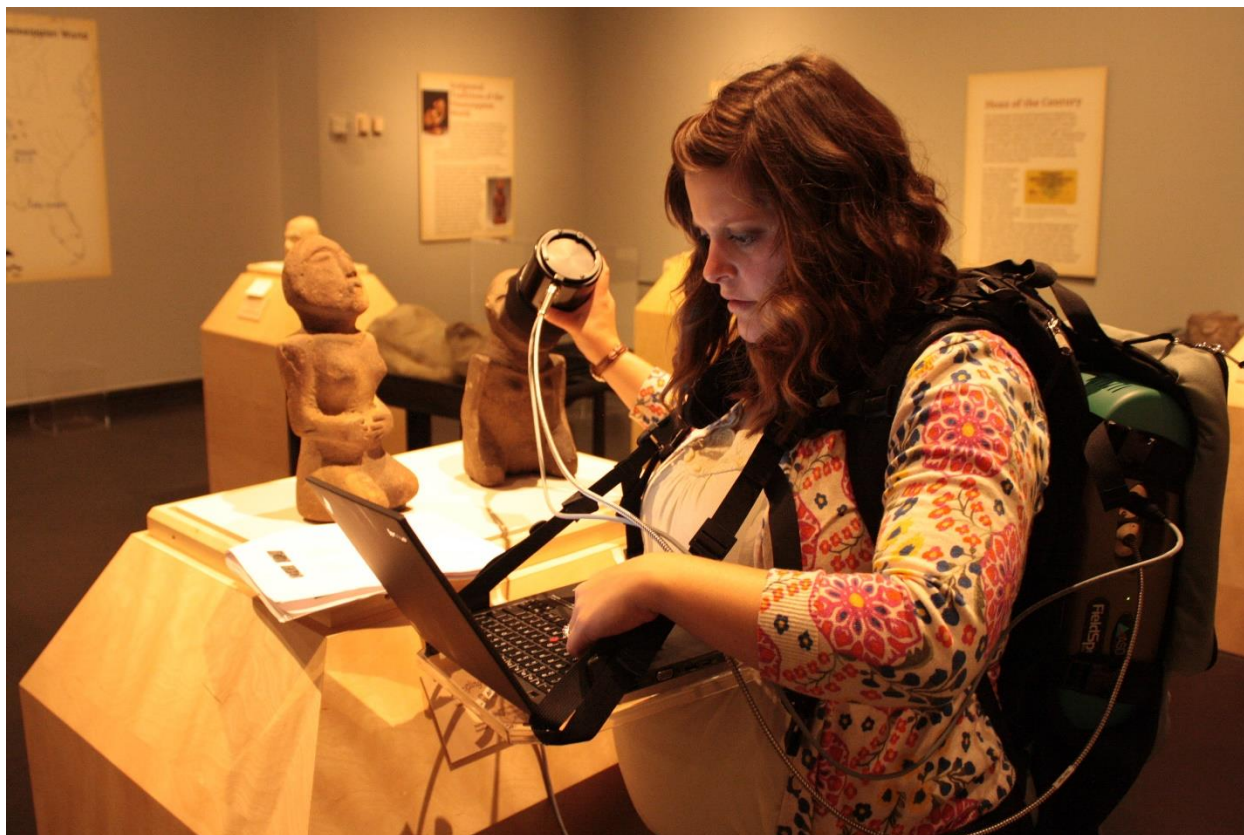
Figure 38: FORS set-up for statuary analysis during the decommission of the exhibit.
