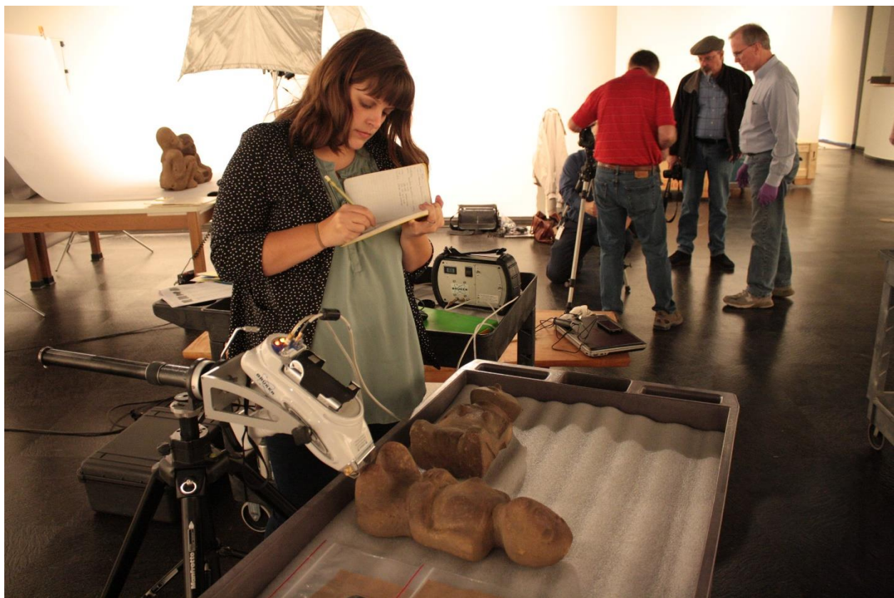
Figure 37: PXRF set-up during the installation of the statuary exhibit.
