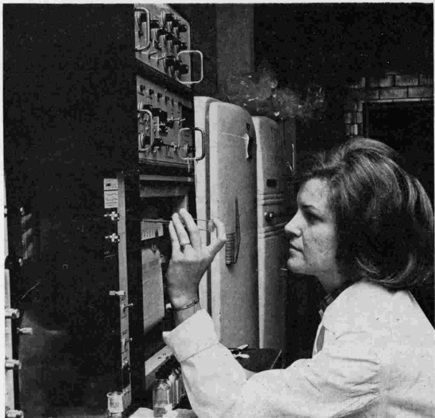
Figure 8. The use of the gas chromatograph has increased the sensitivity of detection of various pesticide residues. Samples of feed, excreta, and milk are extracted and analyzed. A research technician is shown injecting a sample extract in the gas chromatograph for residue analysis.
