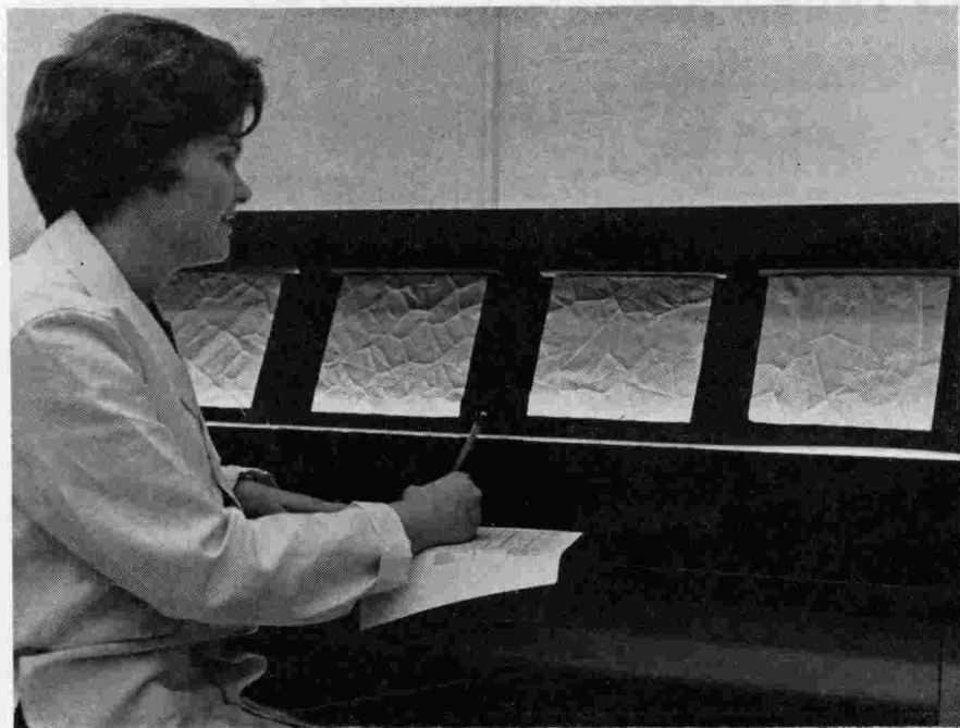
Figure 13. The Celanese Wrinkle Tester. This apparatus is used in evaluating wrinkle recovery of 100% cotton sheeting treated with a permanent press finish. Wrinkles are formed by vacuum action and rated after a standard relaxation time period. This test is one of a series involved in a textile co-operative research project, southern region.
