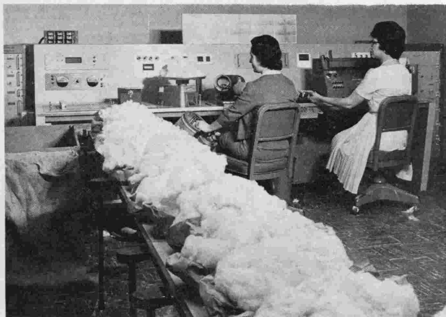
Figure 12. An automated fiber test line at the U. S. Department of Agriculture, Agricultural Research Spinning Laboratory on the agricultural campus. Samples are fed by conveyor belt to two operators who make determinations of color and reflectance on the colorimeter, trash content by inspection, fineness with the speedar, and length with the digital fibrograph. The data from the instruments are fed to a punch for data processing cards.
