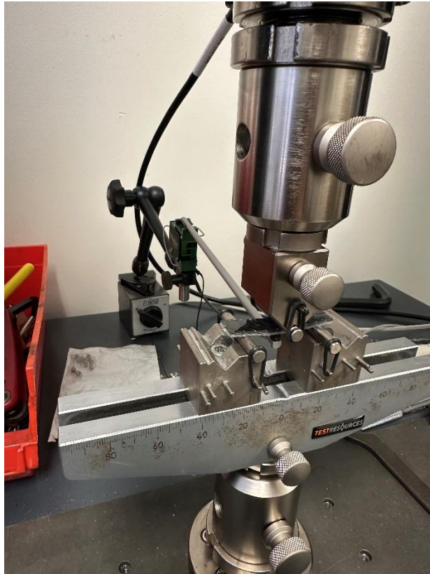
Figure 3.7: Test Resources 3-point bending setup with deflectometer. The composite specimen is supported on two ends (span length) while load is applied at the center. A deflectometer measures the tensile side mid-span displacement to determine flexural properties.
