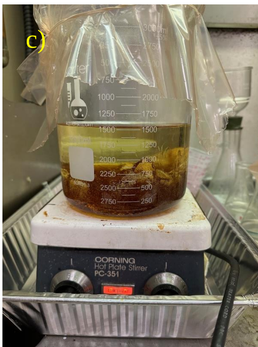
Figure 4.19: Solvolysis of neat EP resin using aqueous acetic acid at 80°C.(a–b) show resin weighing and initial dissolution setup with stirring.(c–d) illustrate resin breakdown and recovered liquid phase for further analysis.
