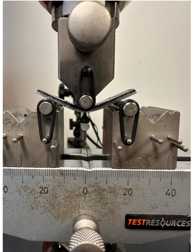
Figure 3.7: Test Resources 3-point bending setup with deflectometer. The composite specimen is supported on two ends (span length) while load is applied at the center. A deflectometer measures the tensile side mid-span displacement to determine flexural properties.
