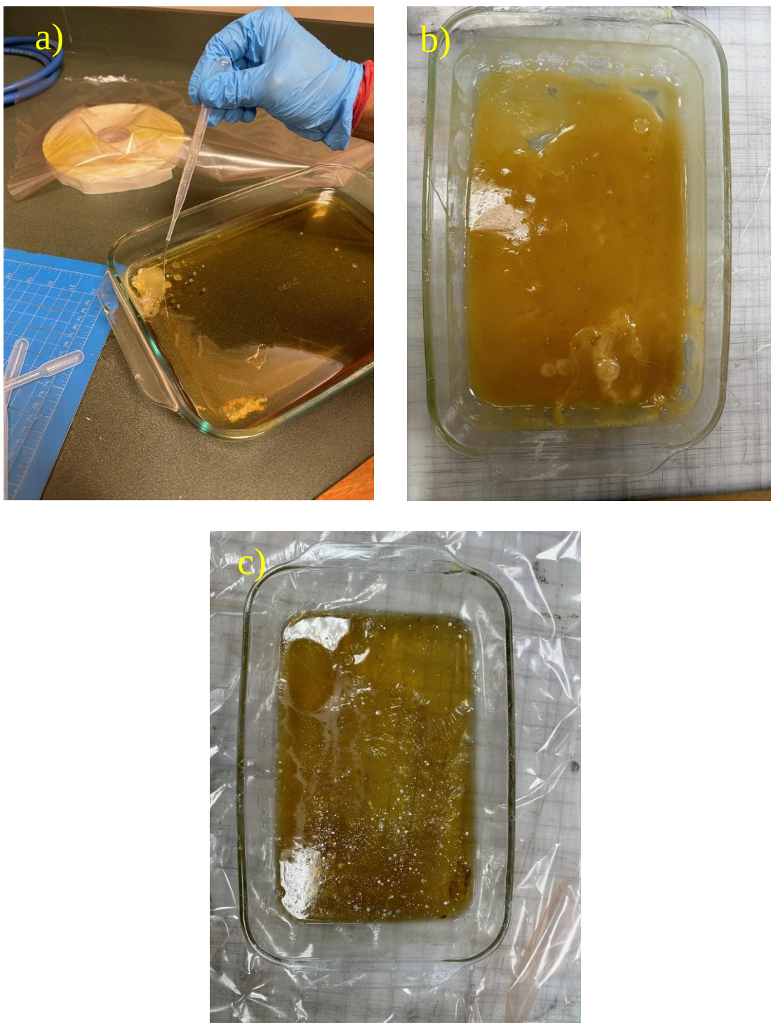
Figure 4.20: Coagulation of solvolized Recyclamine using NaOH neutralization. (a) shows NaOH being added to the recovered solution; (b–c) depict phase separation and coagulated resin. This step enables recovery of the thermoset matrix for potential reuse or further processing.
