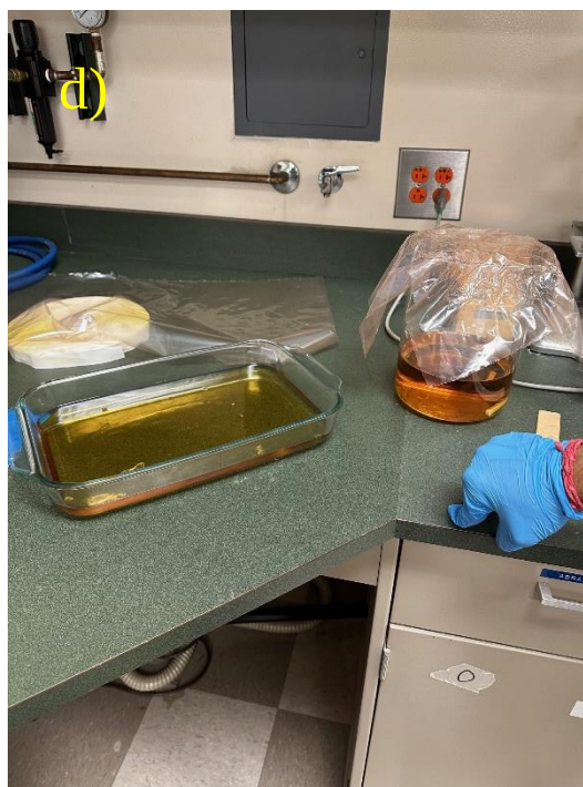
Figure 4.19: Solvolysis of neat EP resin using aqueous acetic acid at 80°C.(a–b) show resin weighing and initial dissolution setup with stirring.(c–d) illustrate resin breakdown and recovered liquid phase for further analysis.
