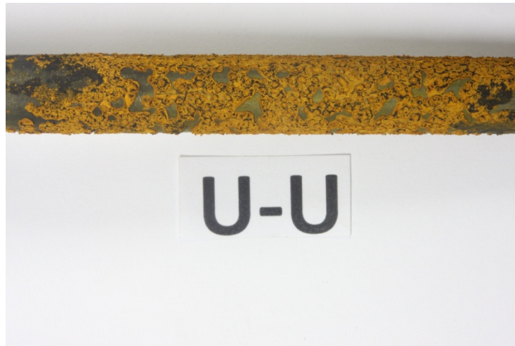
Figure 15: U-U sample has significant rust formation.
