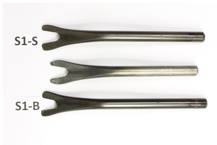
Figure 9: Solution 1 samples showing no rust formation except the lower ring.
