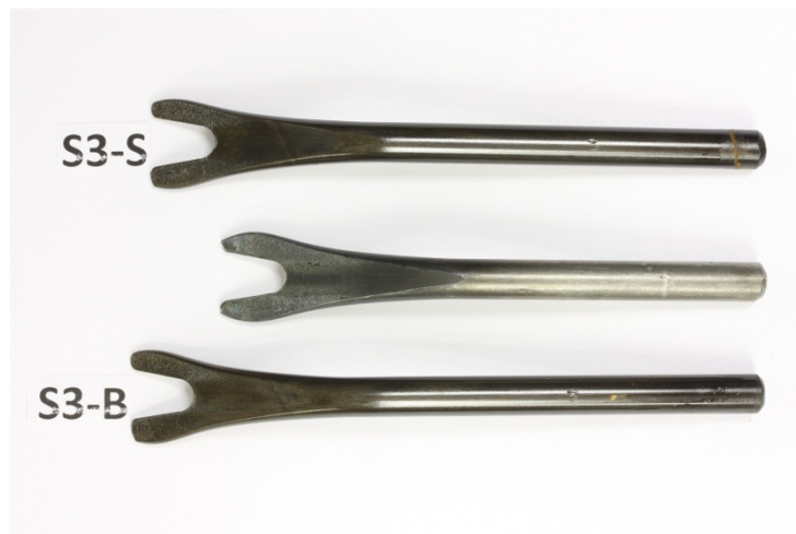
Figure 11: Solution 3 samples have no rust except the ring near the bottom.
