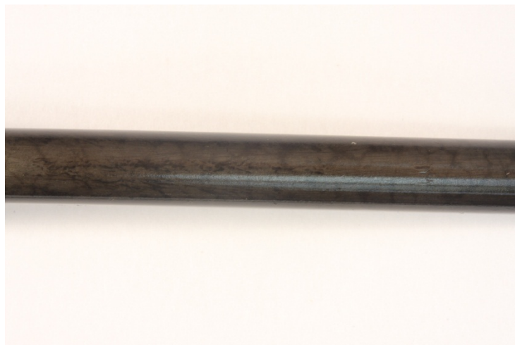
Figure 7: Solution 2, very blotchy thin layer, not a good choice
