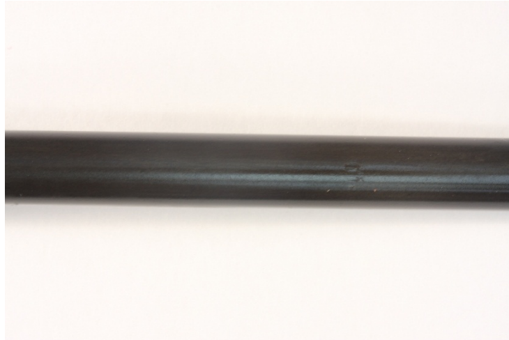
Figure 6: Solution 1, good layer consistency
