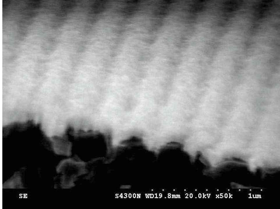
Figure 5.16: Cross-sectional SEM image of sample LL13-3, t_e = 30\text{s} , t_d = 90\text{s} . The interference pattern from the laser interference is barely visible on the surface, suggesting a longer exposure is required. The blurred edges are caused by the 20nm Au conductive coating peeling away from the resist. The sample stage at tilted to 60^\circ . Contrast and brightness has been enhanced in order to highlight faint detail.
