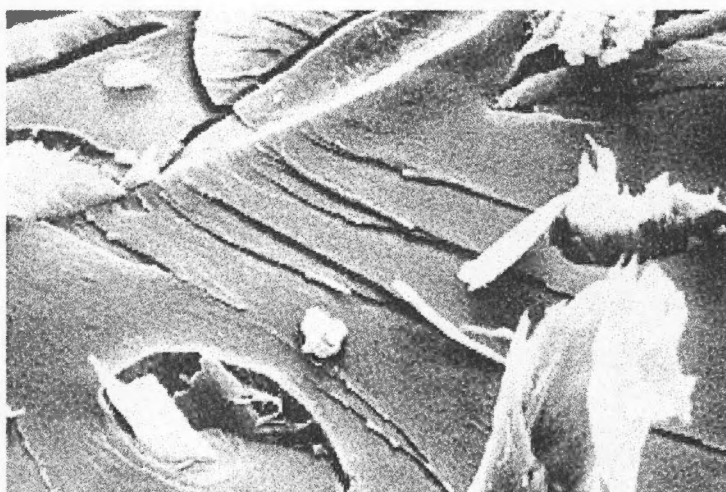
Figure 8. Cotton fiber phenol-Formaldehyde, brittle fracture bands 16
