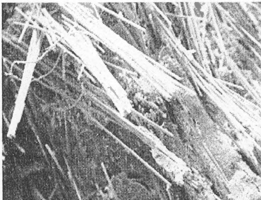
Figure 9. Glass fiber reinforced polyester, fiber breakage and pull-out 16
