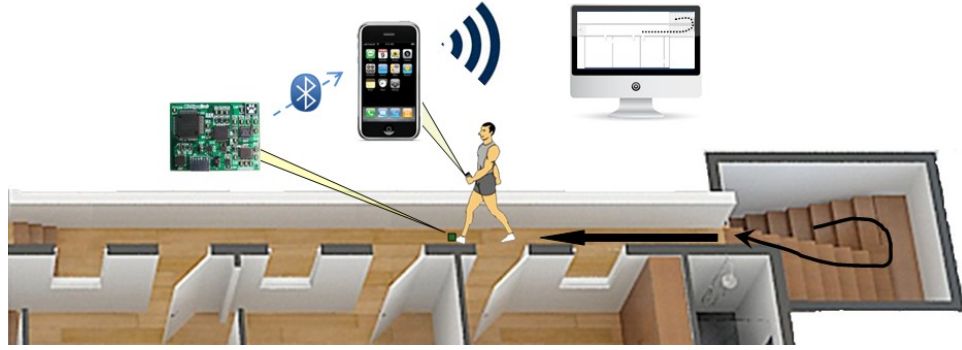
Figure 5.1: A pedestrian positioning system design
