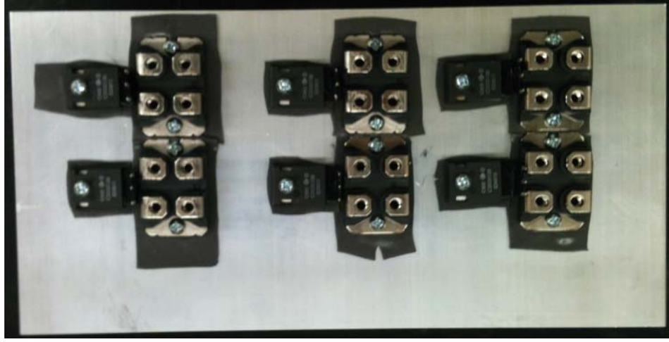
Figure 5.1: Lay-out of the MOSFETs and SiC Diodes.
