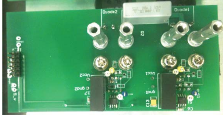
Figure 5.4: Second version of the gate drive circuit.
