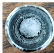
Figure 2.2 - Photos of samples a-d after the crystal growth attempt. Compositions are given in the figure. Compounds did not melt for compositions a) and d) and top view of the \varnothing 16 mm iridium-rhenium crucible with solid material inside is shown. Compounds melted for compositions b) and c) and the grown sample is shown.
