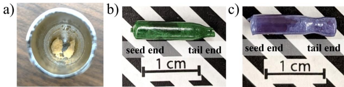
Figure 3.6 - Photos of samples 1, 2, and 3 after the growth attempt. a, Top view of the iridium-rhenium crucible with sintered powder of composition 1 that did not melt at the maximum operating temperature of the crucible. b, Crystal of composition 2. c, Crystal of composition 3.
