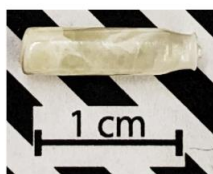
Figure 2.2 - Photos of samples a-d after the crystal growth attempt. Compositions are given in the figure. Compounds did not melt for compositions a) and d) and top view of the \varnothing 16 mm iridium-rhenium crucible with solid material inside is shown. Compounds melted for compositions b) and c) and the grown sample is shown.
