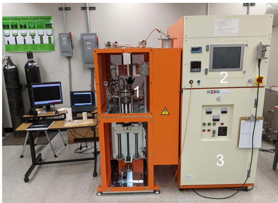
Figure 1.1 - KDN Dai-Ichi Kiden micro-pulling-down growth station installed at the SMRC-UTK. The numbers in the image indicate 1 - the growth chamber, 2 - the control panel, and 3 - the RF generator model TR-02001 operated at 26 kVA.
