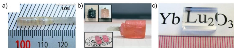
Figure 1.10 - Sesquioxide crystals grown by the mPD method. a) Yb:Y_2O_3 grown by the mPD method [58]. b) Er:Lu_2O_3 grown by the edge-defined film-fed method [64]. c) Yb:Lu_2O_3 grown by the heat exchanger method [69].
