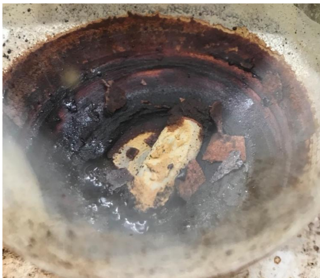
Figure 11. Digestion of Zircaloy® or Zr metal in sulfur monochloride.
