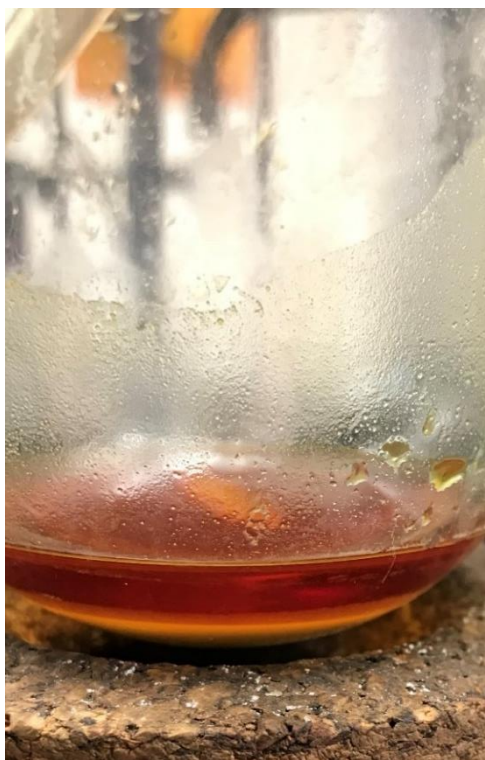
Figure 11. Digestion of Zircaloy® or Zr metal in sulfur monochloride.
