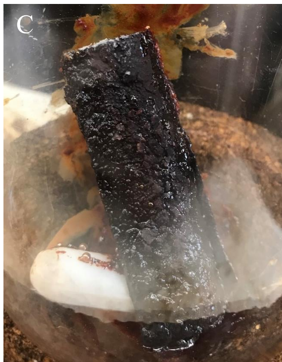
Figure 13. Stages of hydrolysis as a result of degassed water added to flask containing cladding with purple-black layer.
