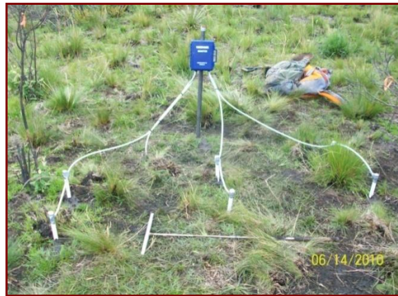
Figure 9 - Datalogger with sensor placement (auger for scale)(photo by author).
