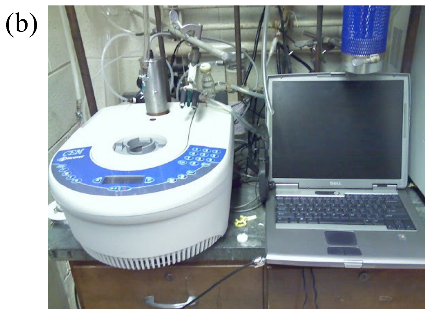
Figure 1.4: (a) Multimode and (b) monomode microwave reactors.
