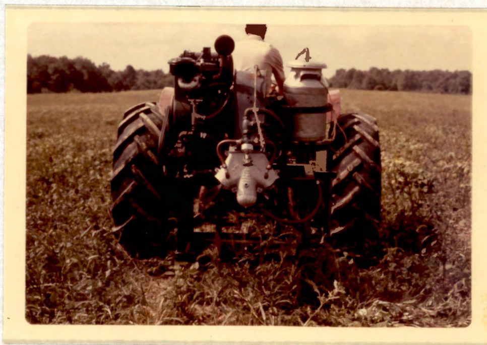
Figure 2. The low-volume John Blue sprayer.
