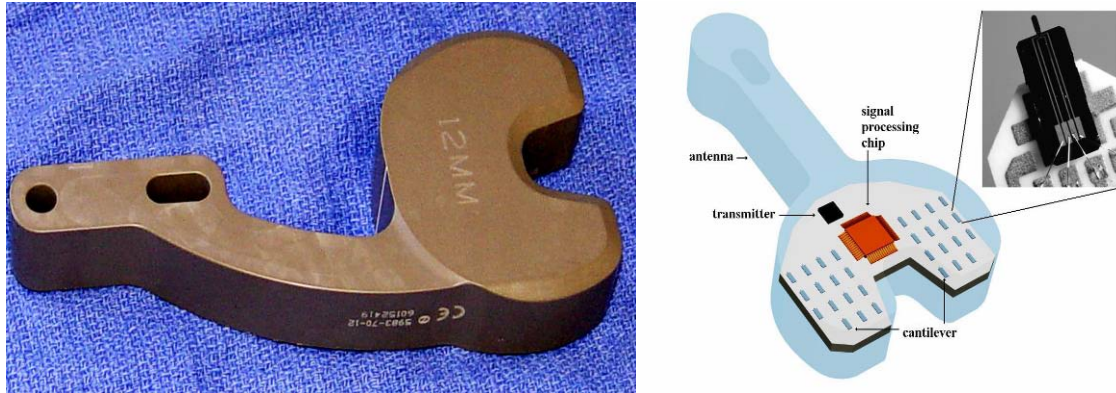
Figure 1.2 Traditional space blocker (left) and newly designed sensor and ASIC technique enhanced space blocker model (right)
