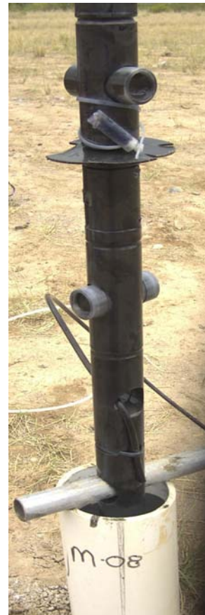
Figure 4-3. Diagram of a Biosep beads sampler (left, also called bio-trap) and multi level samplers (MLS) with bio-traps. Plugs are made of glass wool and the sampler is loaded with Biosep beads.
