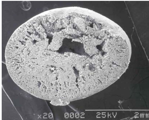
Figure 1-2. Cross section of BioSep® beads, 2-3 mm in diameter, autoclavable. 74% porosity, 600 m 2 of surface area/g, 25 % Nomex, 75% Powdered Activated Carbon [PAC], Surrounded by ultrafiltration-like membrane with 1-10 micron holes, Cleaned of contaminating biomarkers by heating to 300 °C 5 hrs.
