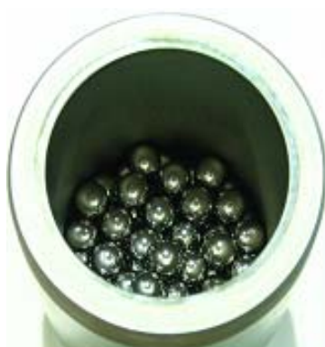
Fig. 22 (b) Stainless steel vial and stainless steel grinding balls
