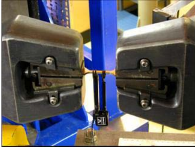
Fig. 29 Wedge grips and flat tensile specimens used in ENGIN-X
