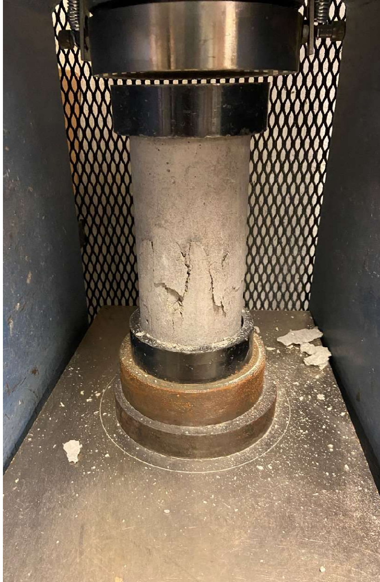
Figure 4-43: A-LS1-MS-0 Post-Compression After 600°C Heating
