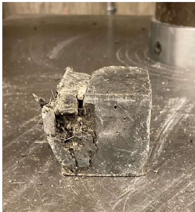
Figure 4-26: 14 Day Composite Specimen Post-Compression (Elevation View)
