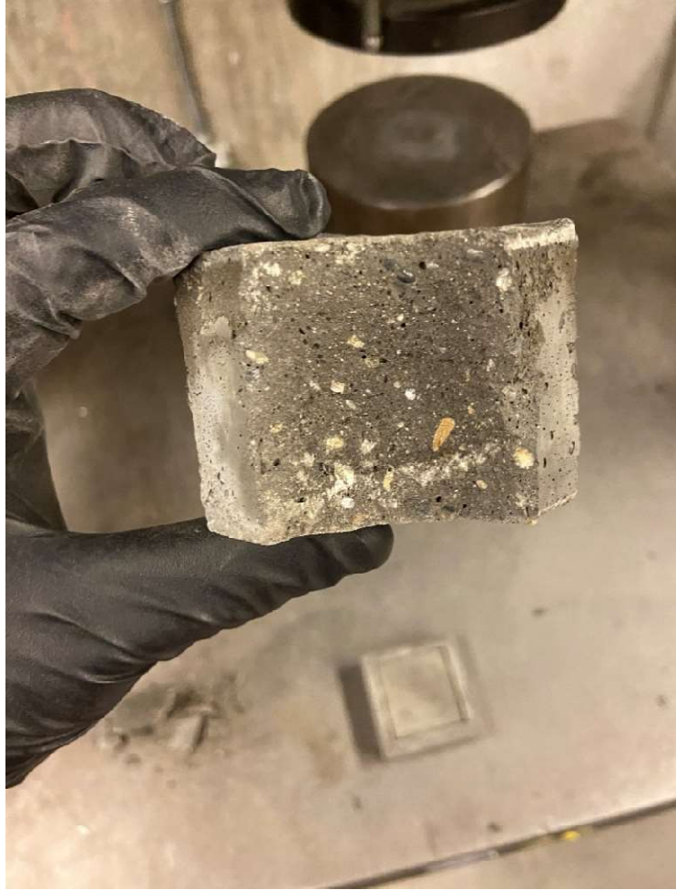
Figure 3-2: Failed Matrix Specimen Interior
