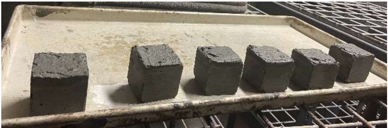
Figure 4-18: Well-Compacted Matrix Samples
