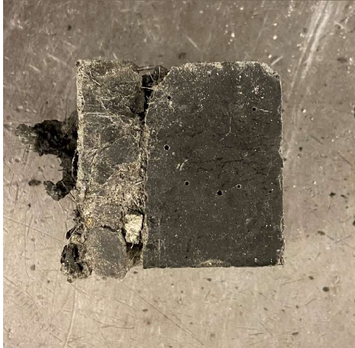
Figure 4-27: 14 Day Composite Specimen Post-Compression (Plan View)
