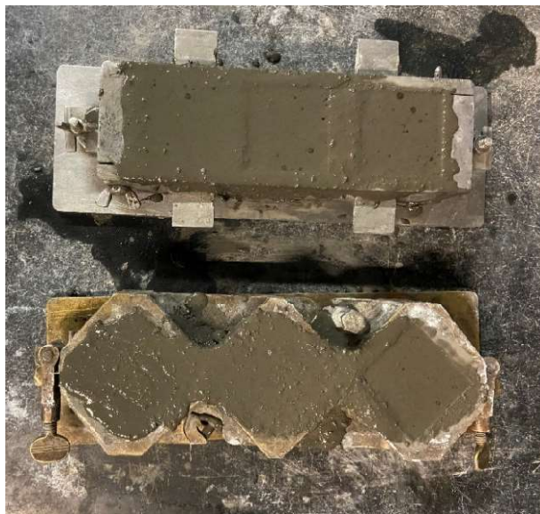
Figure 4-24: Fresh Composite Cubes
