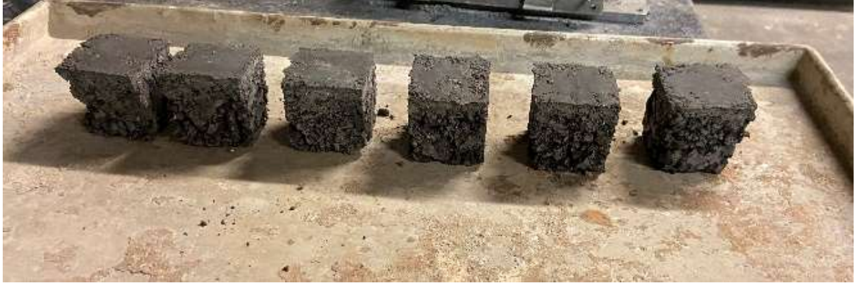
Figure 4-19: Poorly-Compacted Matrix Samples
