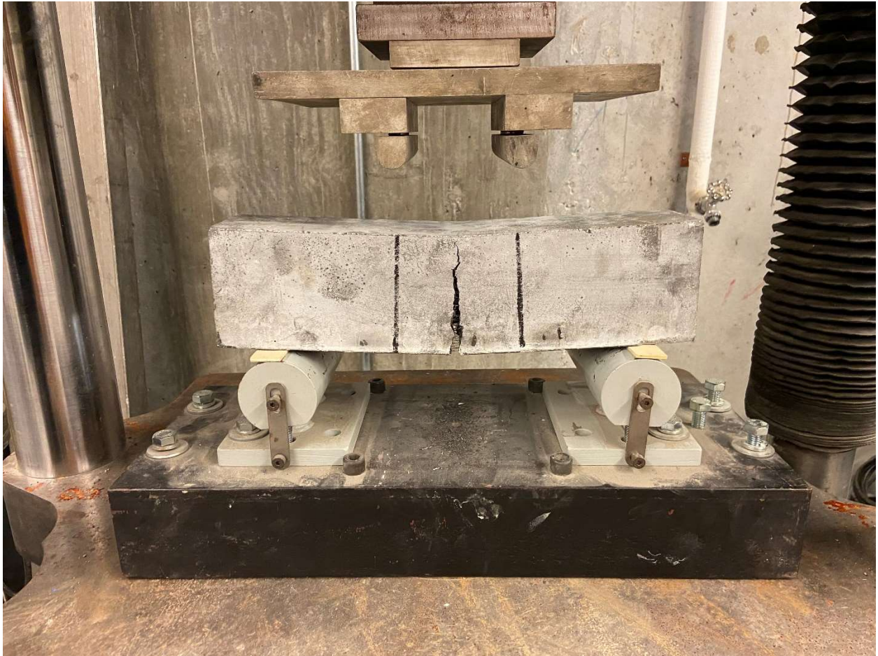
Figure 4-38: Flexural Test Loaded to Fiber Separation
