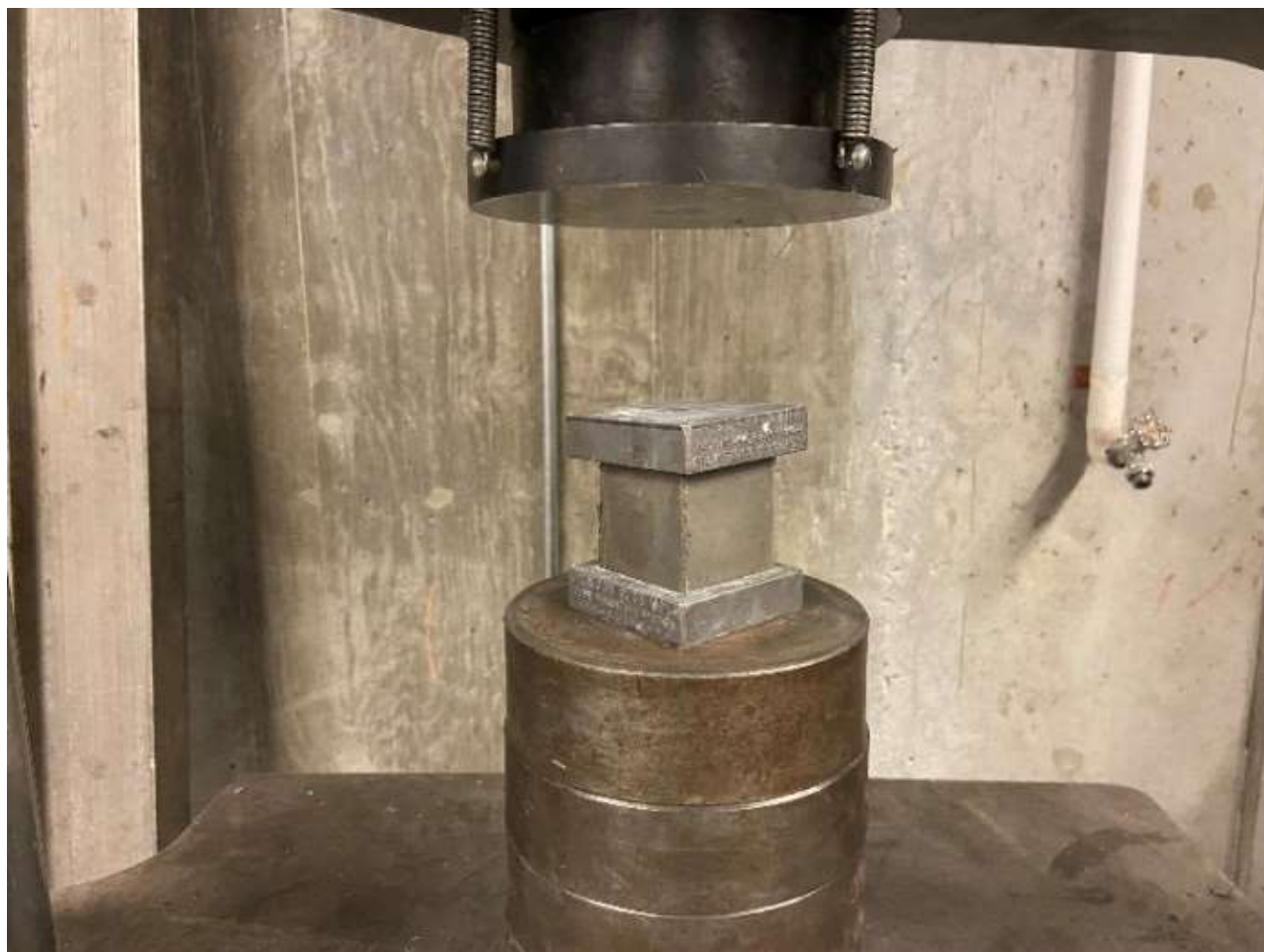
Figure 4-11: Matrix Compression Setup
