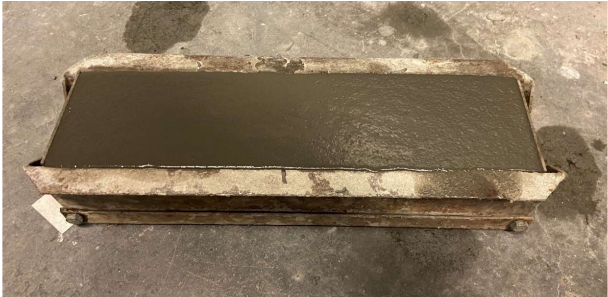
Figure 4-34: Fresh UHPC Flexural Specimen
