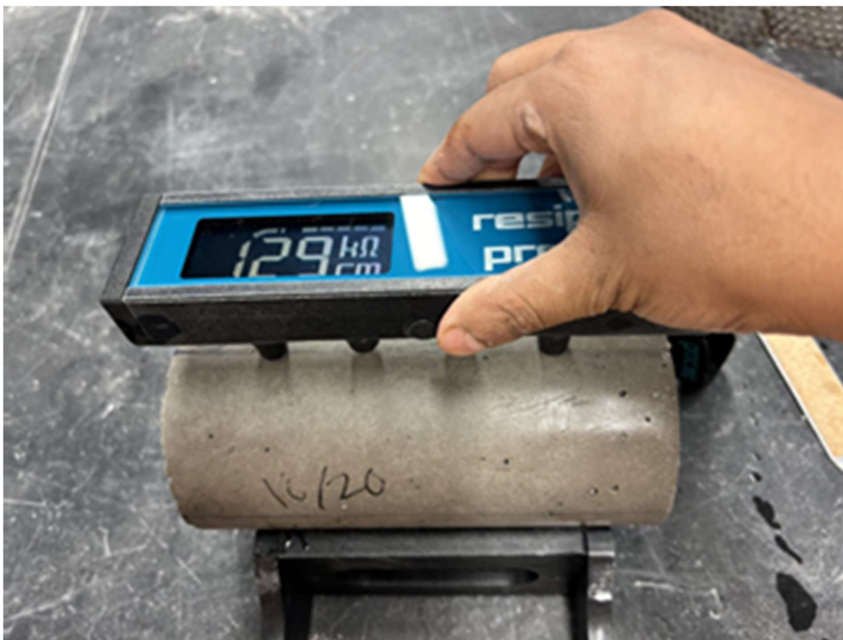
Figure 4-3: Surface Resistivity Testing In-Action
