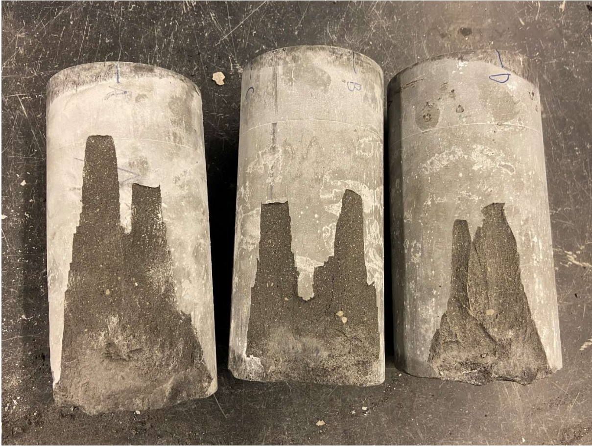
Figure 4-17: Cylindrical Matrix Cracking Pattern
