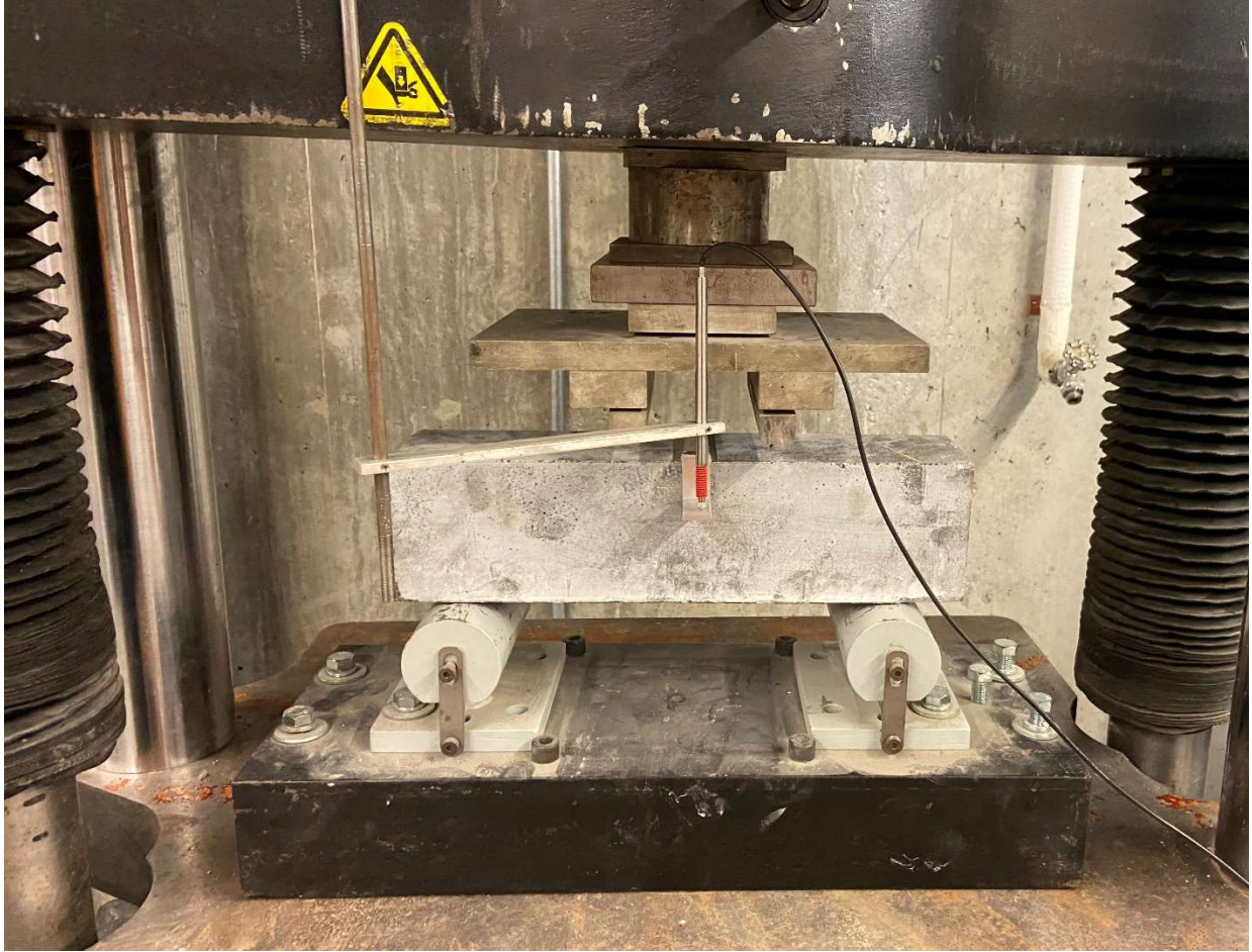
Figure 4-36: Flexural Test Configuration
