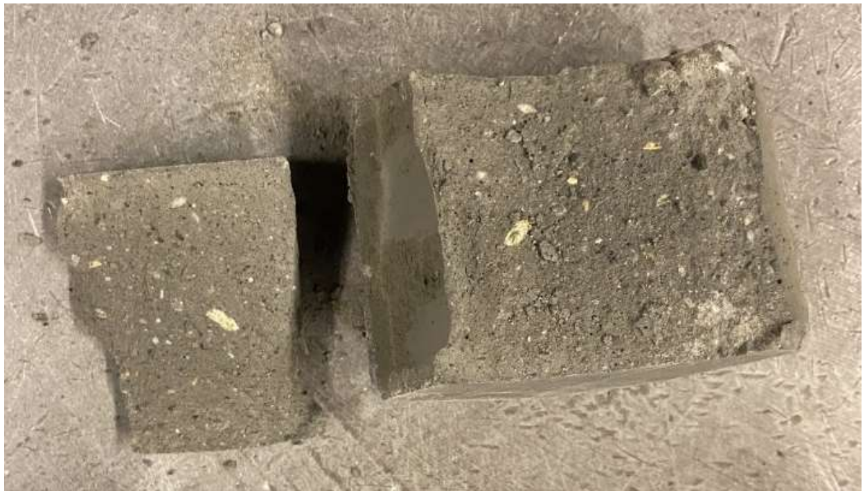
Figure 4-20: Cracked Matrix Specimen
