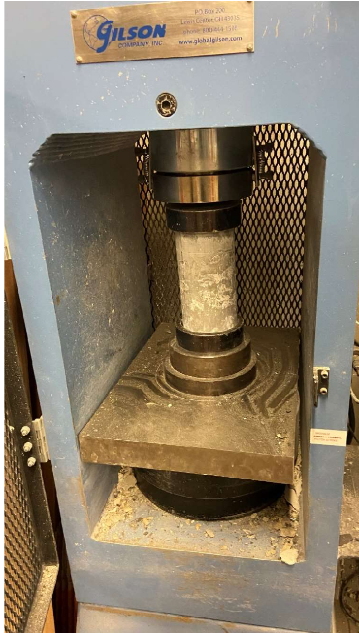
Figure 4-15: Cylindrical Matrix Compression Setup
