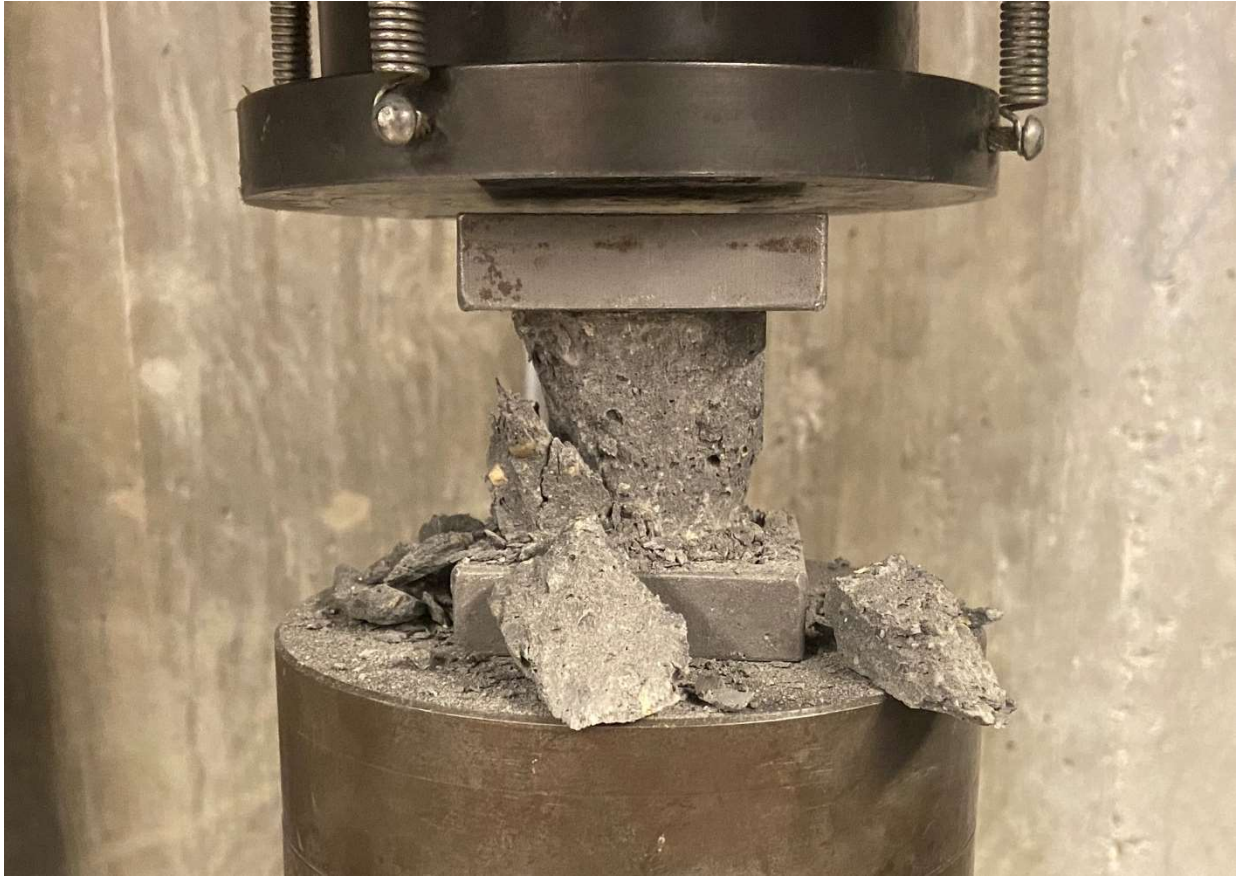
Figure 4-14: Failed Matrix Specimen in Instrument
