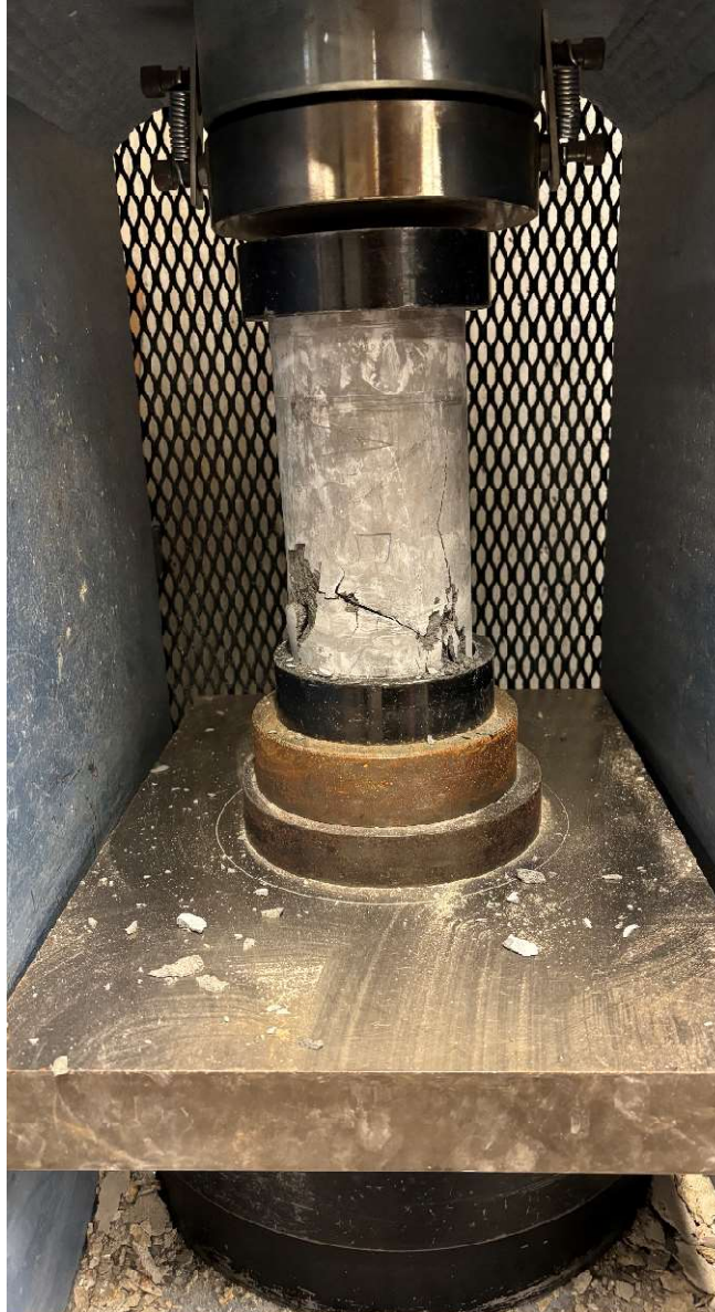
Figure 4-44: Ac5 Post-Compression After 600°C Heating
