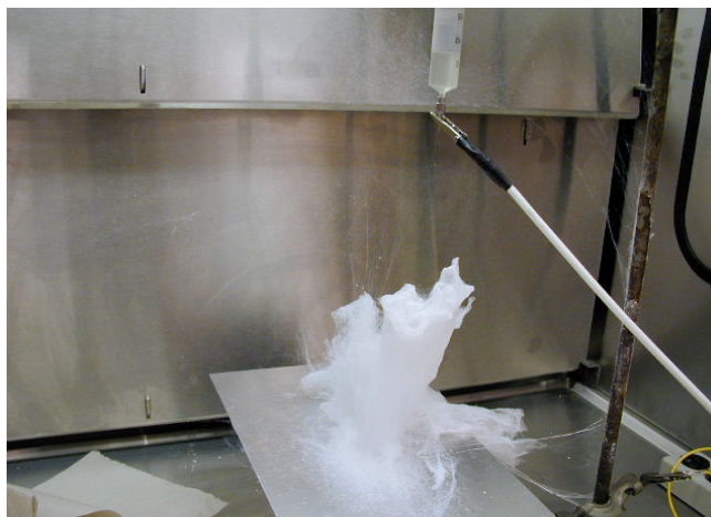
Figure 5 The Electrospinning Process in Action
