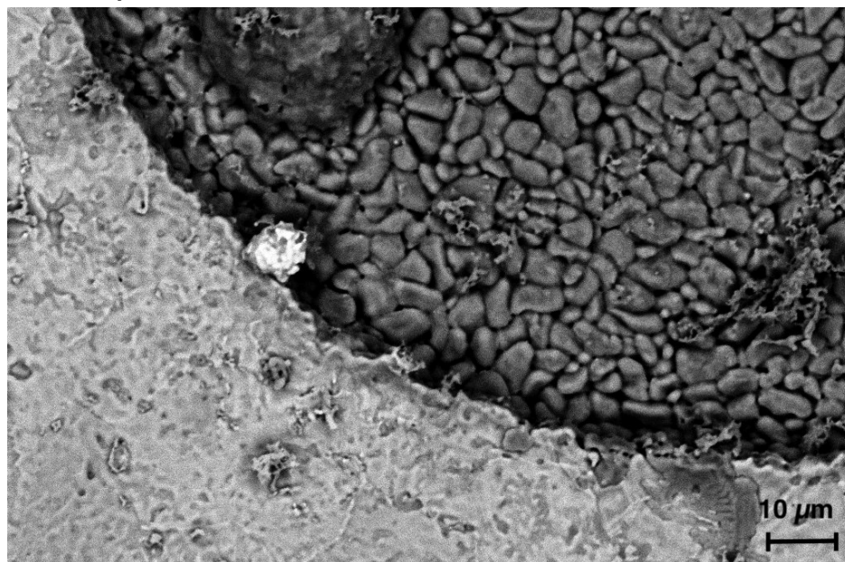
(a) BSE image of significant ZrO 2 deposition region in 60 vol% after 4 thermal cycles at 2000 K.
