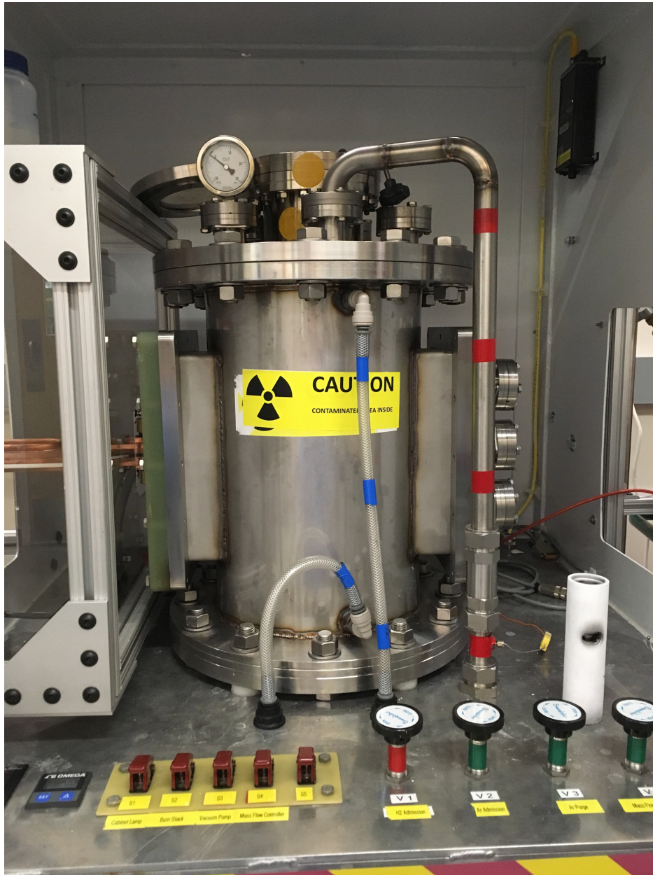
Figure 4.4: The Compact Fuel Element Environmental Test (CFEET) facility at NASA Marshall Space Flight Center
