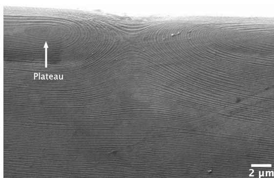
(d) Plateaus in the Mo near the edge of the sample surface
