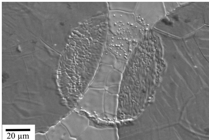
(a) Secondary electron (SE) image of small \text{ZrO}_2 deposition region of the 60%YSZ sample under thermal cycling at 2250 K.
