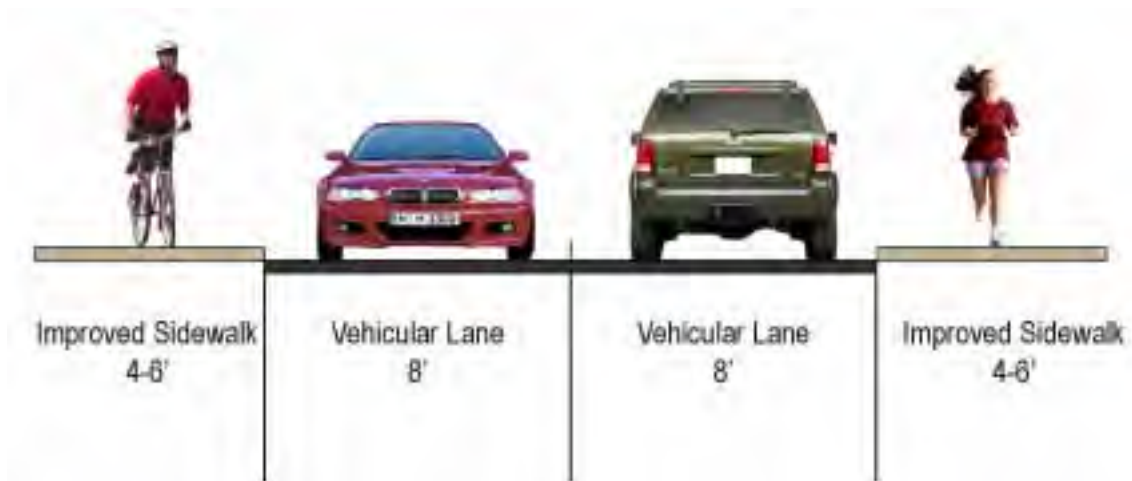
Figure 24: Section showing proposed shoulder improvements
