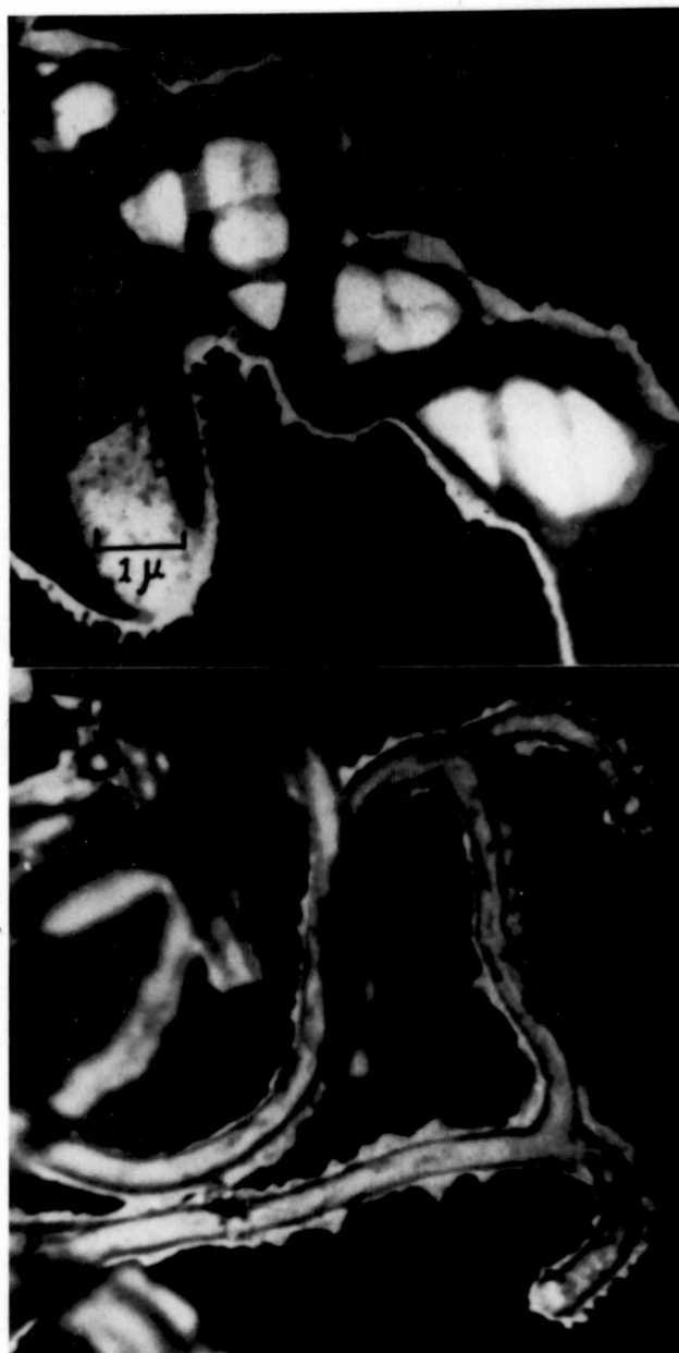
Figure 3.1. Images produced by Locquin that are believed to be the first electron micrographs produced using a phase plate.
