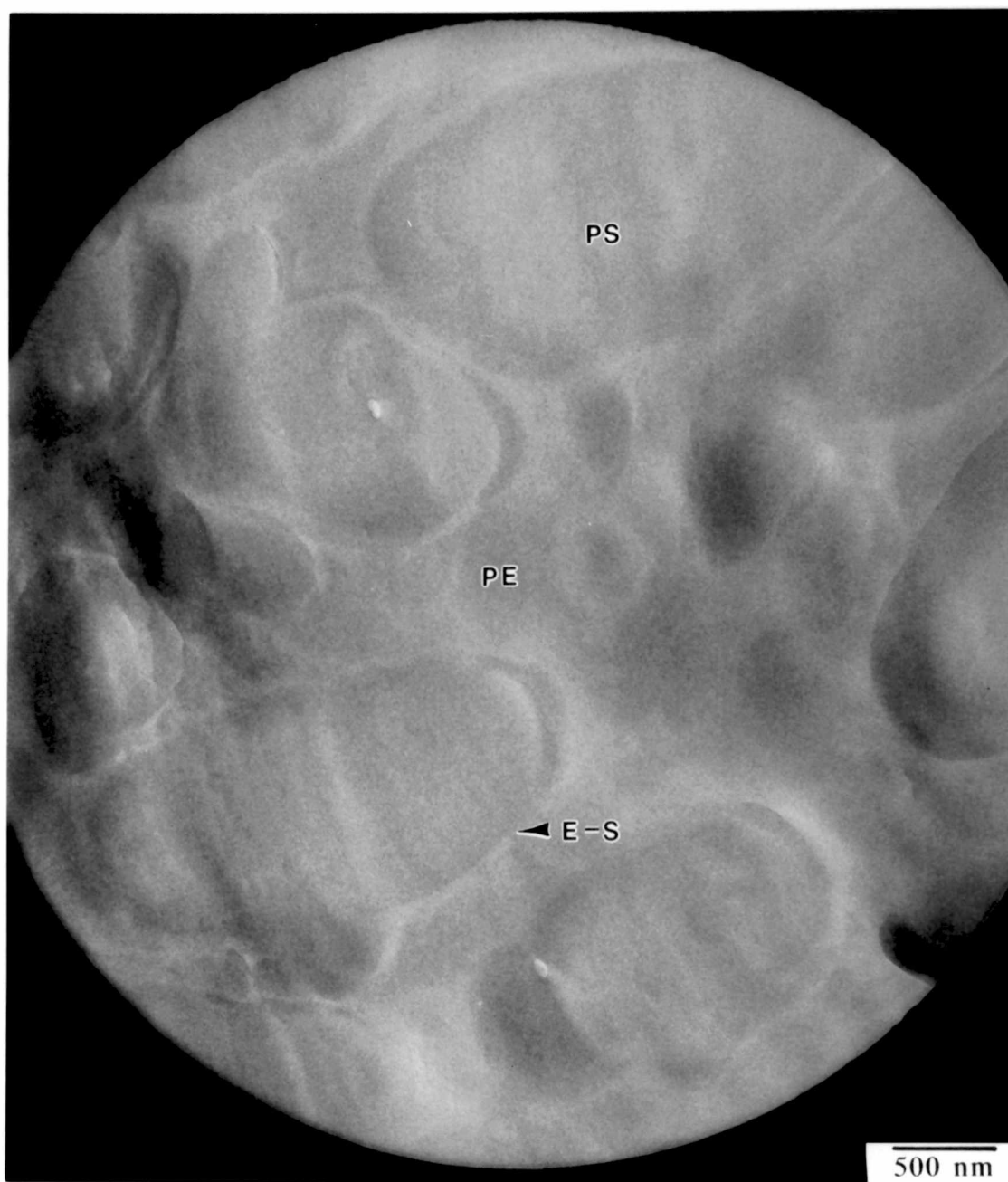
Figure 6.26. A TEM micrograph of an unstained, ultramicrotomed thin section of PS/PE/E-S copolymer taken using a 75 \mu\text{m} objective aperture, a 100 \mu\text{m} condenser aperture, a #2 CL1 setting and an objective lens approximately -38.8 nm defocused.
