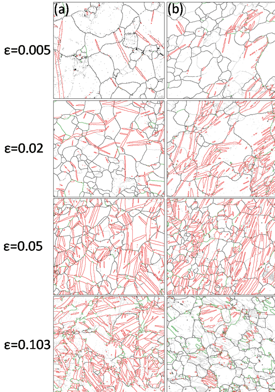
Figure 6-7 Boundary map with various strain under the tension along ND ( c -tension) and compression along TD ( a -compression) obtained through EBSD: (a) c -tension and (b) a -compression.
