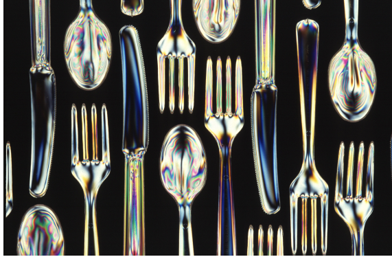
Figure 2: Stress Picture by Transmission Polarization
