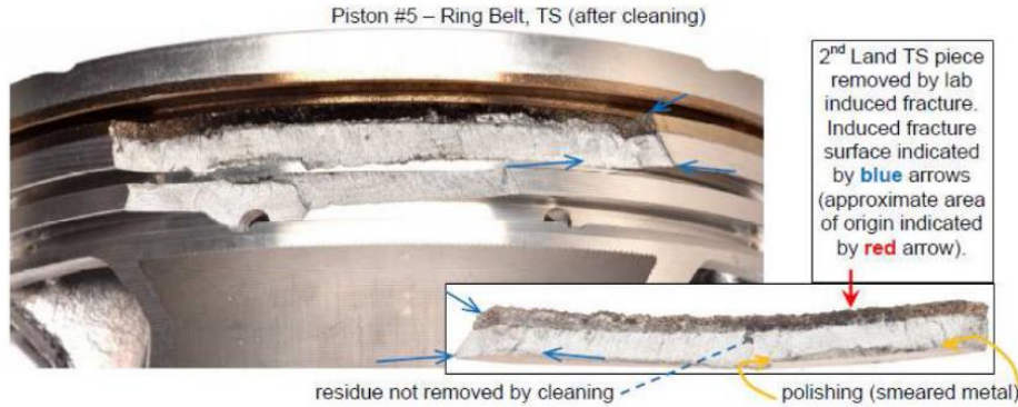
Figure 2 A damaged ring carrier piston following a severe LSPI event in a downsized turbocharged spark-ignited engine that fractures the second ringland. From Passow et al. [8]
